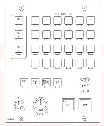
SELECTOR 3: 24 Stereo external inputs. Green LEDs.
