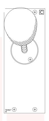
For those customers requiring a microphone projecting from the console on a stalk.
