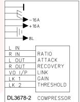
The compressor and limiter normally respond to the higher of the left and right signals. An internal option allows the mono reduction of left and right (-3dB) to take control if the Stereo coherence is such that this exceeds left or right. This renders it unnecessary to "under-drive" the stereo outputs to guard against the possibility of a higher than desired mono level.
