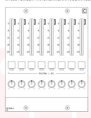
Each Bargraph Control panel provides control over 8 tracks. The Bargraph Meters are GREEN from -oo to -6, YELLOW from -6 to 0, and RED from 0 to +6. There are usually 3 panels for 24 tracks and 4 for 32 track systems.
