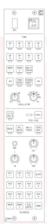
Master AFL indicator illuminates Red when any AFL button is selected or a multitrack AFL is switched in. Also illuminates AFL LED on ML4230 Monitor Loudspeaker panel.
