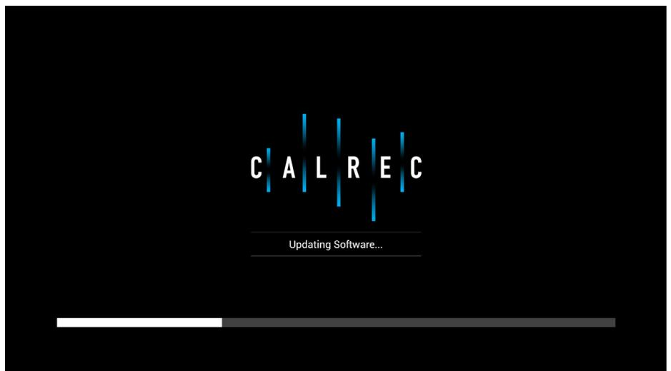
If a long reset was required, once it is complete, the green 'success' icon will be displayed across the surface and you should perform a short reset by simply tapping the Surface Reset button once. If any surface sections fail to update, retry another long reset.
