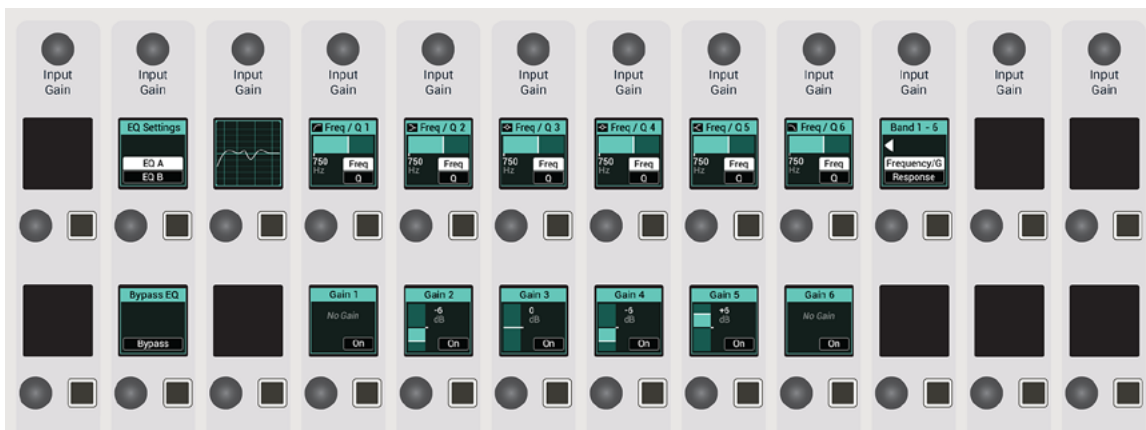
FIGURE 1 - CONTROL CELLS—ACCESS MODE—EQ
