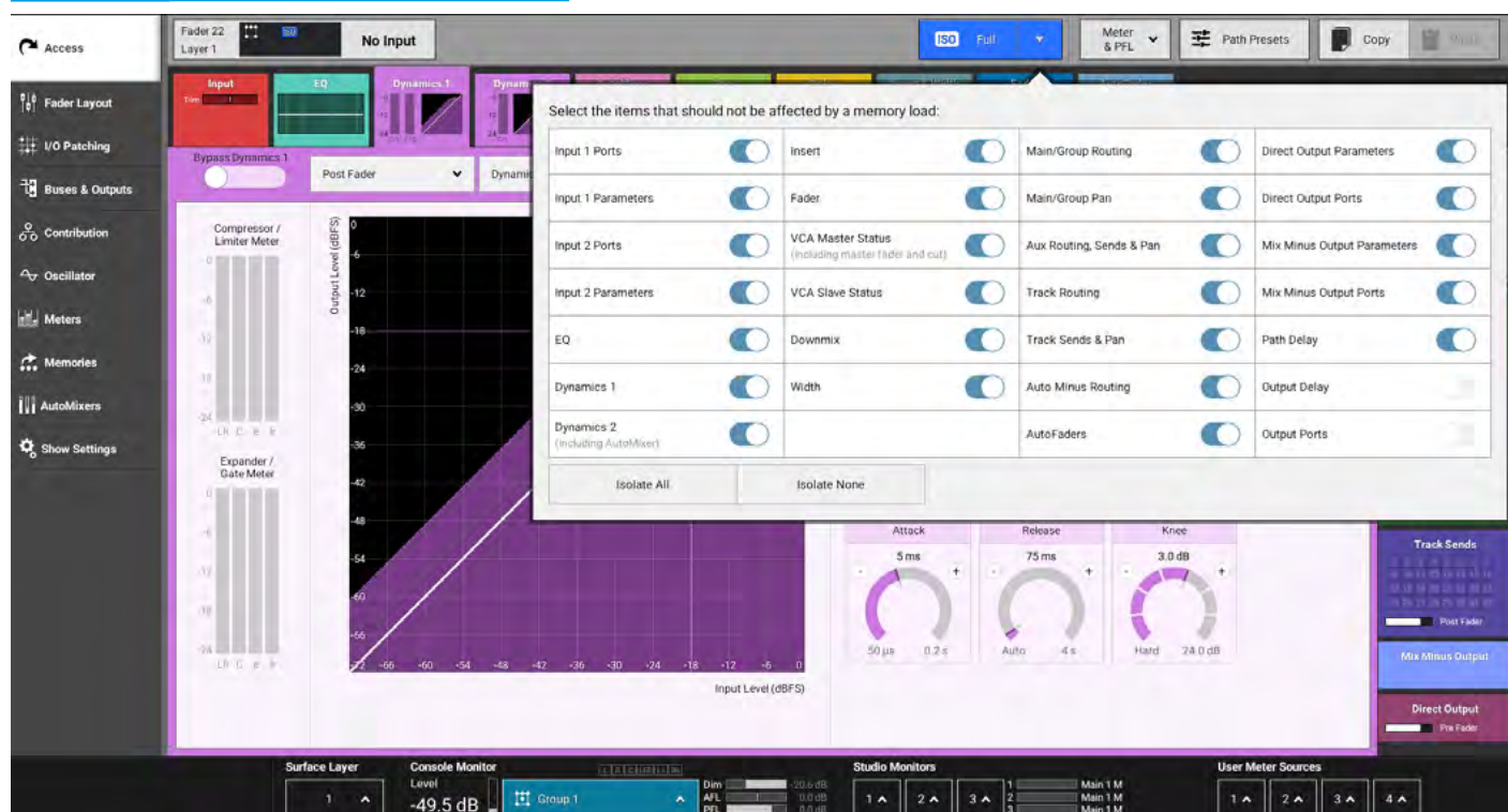
FIGURE 4 - ISOLATE SELECTOR WINDOW
