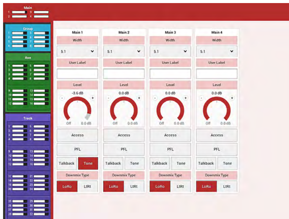
FIGURE 2 - ROUTING TONE TO A BUS OR OUTPUT
