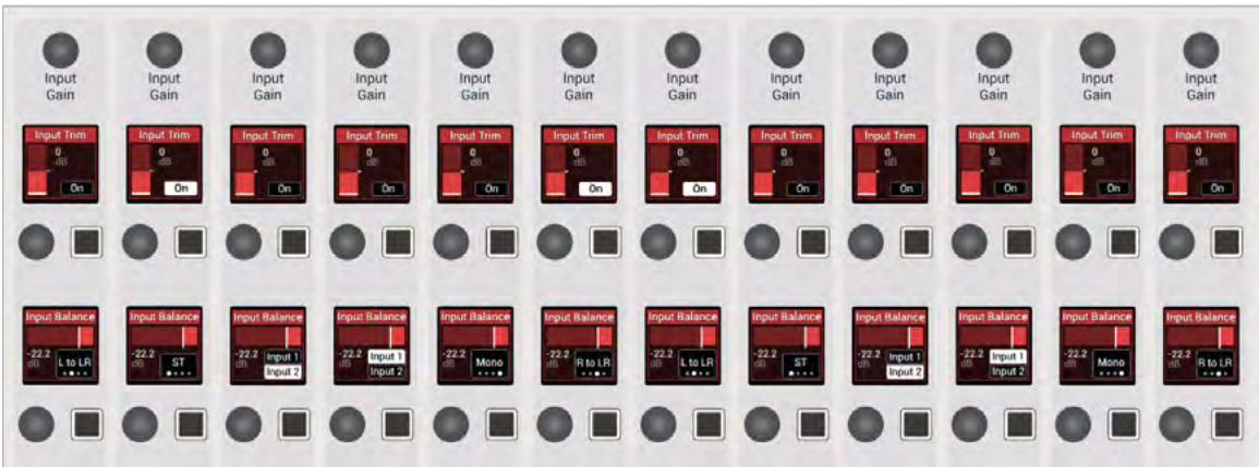
FIGURE 2 - CONTROL CELLS—INPUT CONTROL MODE
