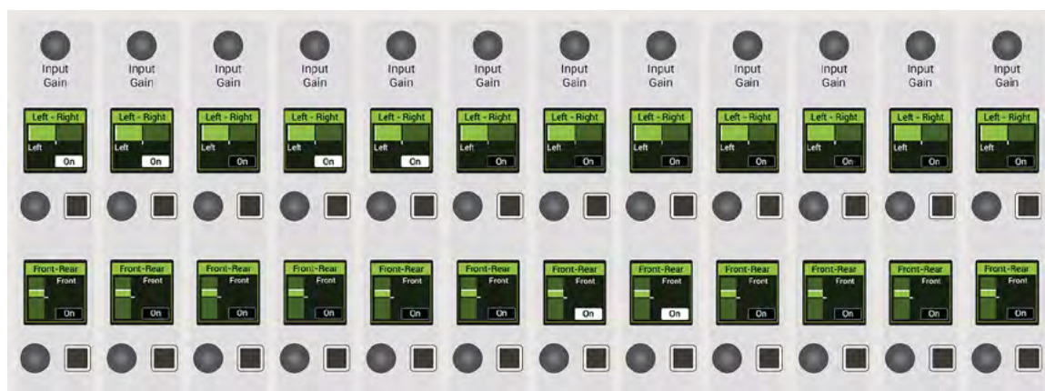
FIGURE 2 - CONTROL CELLS IN PAN CONTROL MODE
