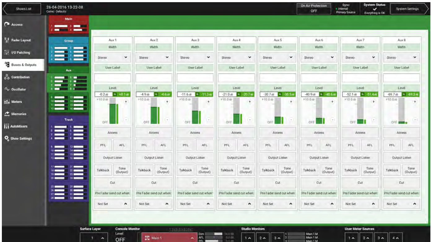
FIGURE 4 - AUX BUS OUTPUT FADERS—SLAVES IN VCA GROUP
