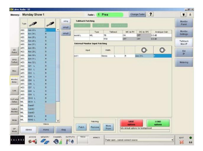
The input sources for Talkback, Reverse Talkback and the external monitor input are patched on this screen. This screen is only visible in engineer mode.
