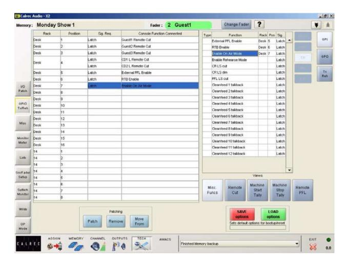
The Tech - GPIO TX/REH - GPI screen allows the system's 32 opto-isolated general purpose inputs to be set up. This screen is only visible in engineer mode.
