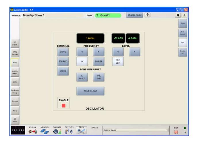
This screen provides controls for the oscillator, which is used to generate test tones for alignment and testing. This screen is only visible in engineer mode.
