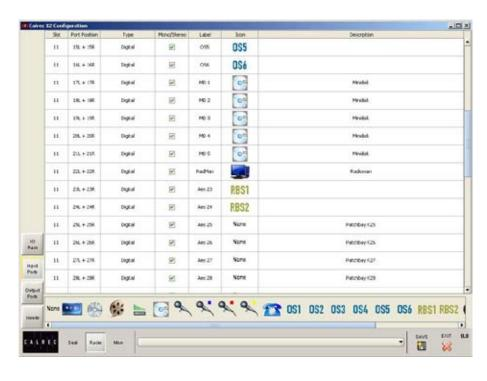
A mono channel input or direct output can be connected to any of: The L or R of a pair of ports, or any mono port.
