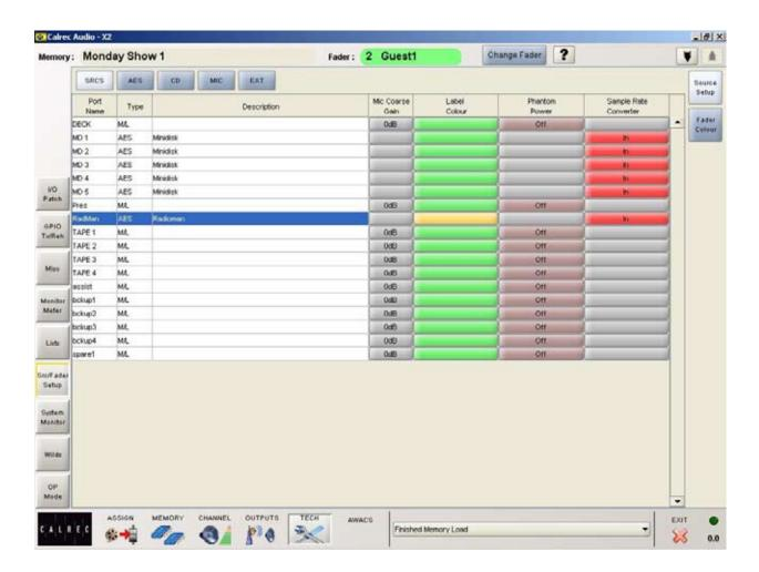
This screen allows the user to set the following functions for each input source. This screen is only visible in engineer mode.
