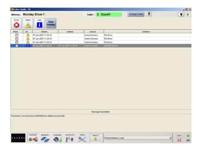
If a problem does develop, messages are delivered on the Automatic Warning and Correction System (AWACS) screen.
