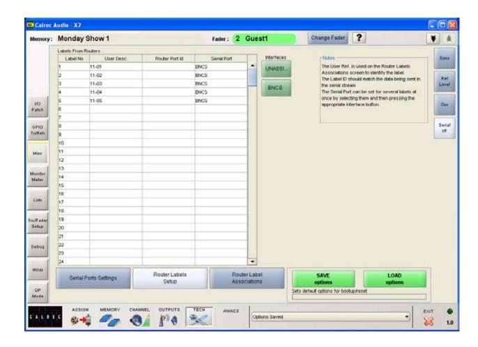
Some Routers incorporate a label interface which is used for the transmission of source (input) and destination (output) descriptions between itself and other equipment.
