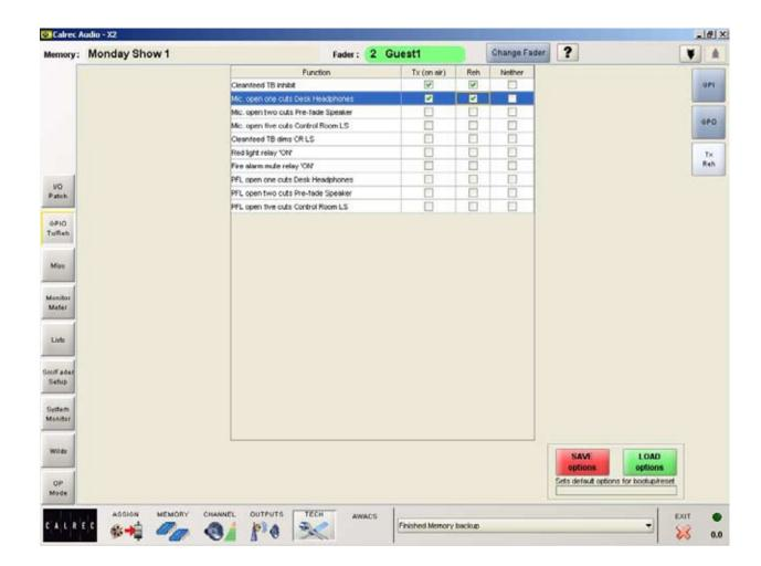
This screen provides a mechanism for the system's condition switching to be set up. This screen is only visible in engineer mode.
