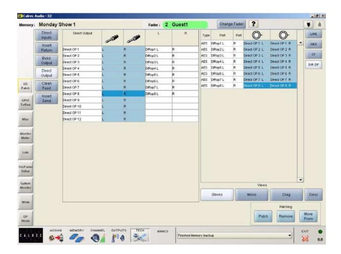
The Tech - I/O Patch - Direct Output screen allows patching of direct output signals to output ports. This screen is only visible in engineer mode.
