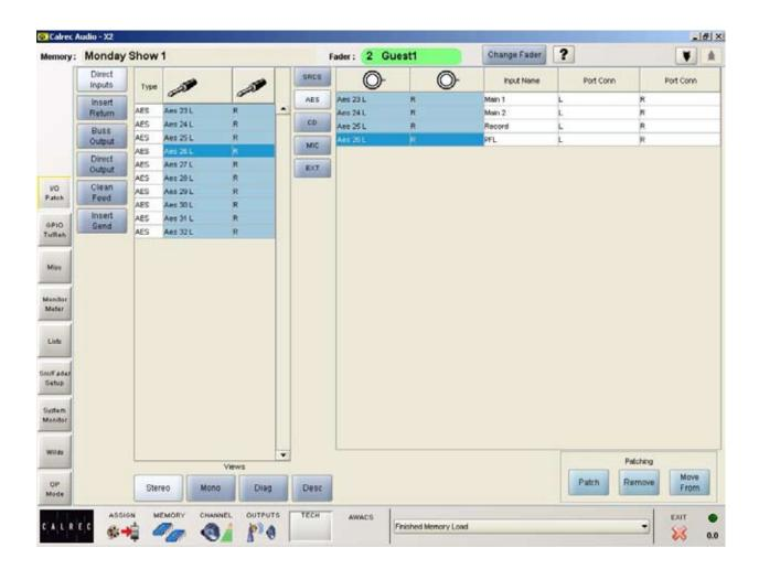
The Tech - I/O Patch - Direct Input screen allows patching of input ports to main, record and PFL direct inputs. This screen is only visible in engineer mode.
