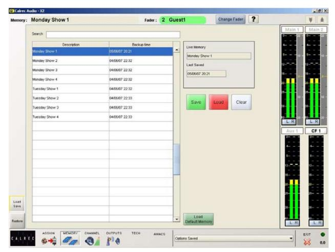
The memory system allows the user to save different console arrangements. This can be useful when many different operators use the same console, or when the console is used to broadcast many different weekly productions. The Memory - Load Save screen is used to load and save memories,
