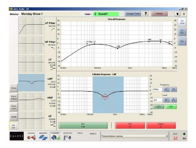
This screen controls EQ and Filters on the currently assigned channel. The user can view and manipulate the EQ and filter response curves, using the touch screen.
