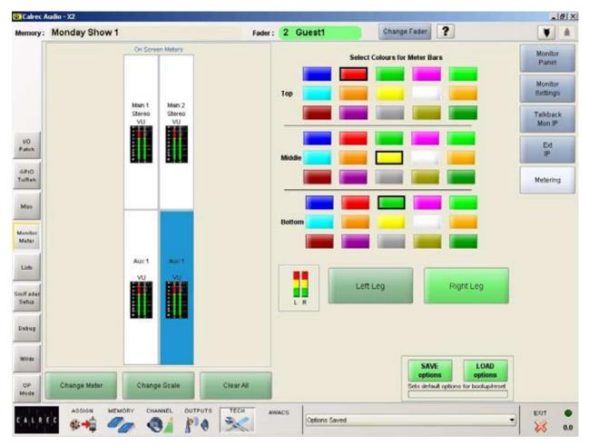
This screen allows the user to change settings for the 4 screen based meters.
