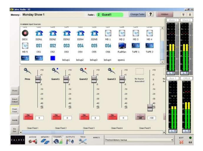
This screen is used to control up to 30 mono clean feed outputs. Each clean feed is fed with all channels routed to the mix minus bus, minus the source it is feeding.
