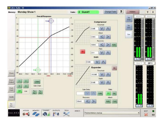
This screen controls the compressor/ limiter and expander/gate on the currently assigned channel.
