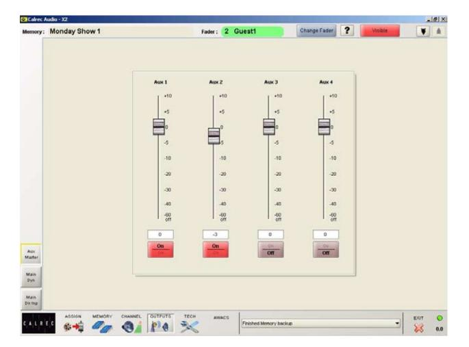
The master send levels and On/Off switching for the 4 stereo auxiliary outputs are available on this screen.
