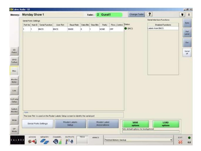
The console has a serial interface port on the rear of the console processing unit to allow the console to be connected to a BNCS (Broadcast network Control System). The Misc - Serial I/F screens provide controls to set up the console's serial port and any router label associations. This screen is only visible in engineer mode.
