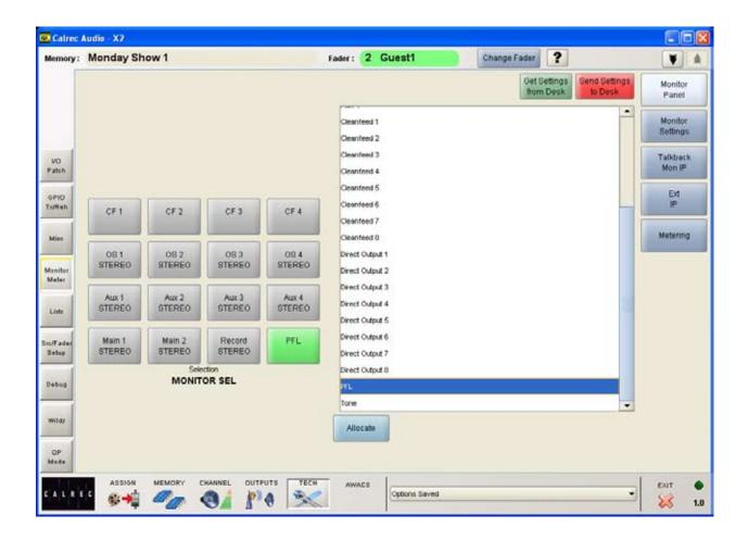
This screen allows all the available monitor sources to be allocated to the 16 selection buttons on the monitor panel. This screen is only visible in engineer mode.
