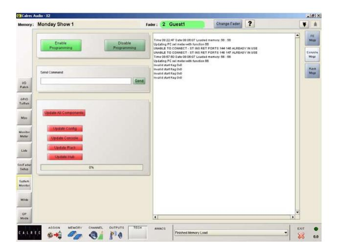
This screen logs system messages, allows debugging and system updates to be carried out. They allow a Calrec support engineer to update and troubleshoot your system. This screen is only visible in engineer mode.
