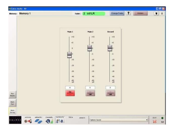
The direct input levels and On/Off switching for main 1, main 2 and record are controlled using this screen.
