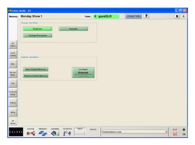
The console can be in one of two operational modes, "Operator", or "Engineer". Operation of certain screen functions is only available in "Engineer" mode, which is password protected to add an extra layer of security. The Tech - OP Mode screen is used to log in and out of different modes.
