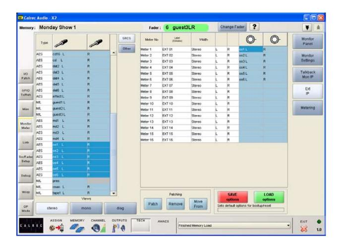
The input sources for external meters can be patched on this screen. There can be up to 16 mono or stereo external meter inputs. This screen is only visible in engineer mode.
