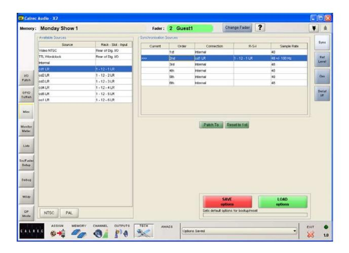
The Misc - Sync screen allows the system's synchronisation sources to be set. This screen is only visible in engineer mode.
