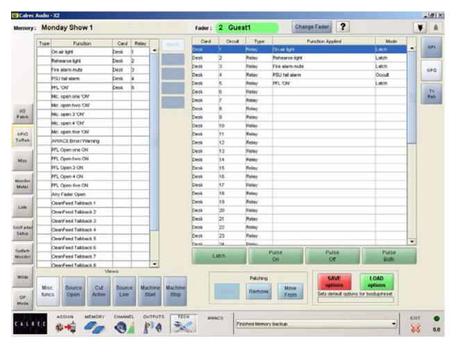
The GPO screen allows the system's 48 relay-isolated general purpose outputs to be set up. This screen is only visible in engineer mode.
