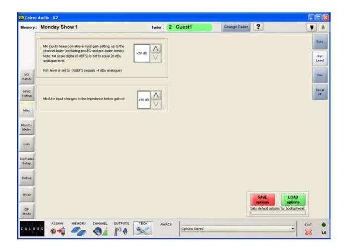
The Misc-Ref Level Screen allows the following console functions to be set. This screen is only visible in engineer mode.
