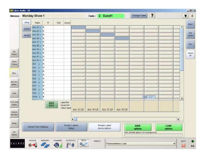
The Tech - Misc - Serial I/F - Router Labels Associations screen allows each of the defined labels to be associated with one of the console's input ports.
