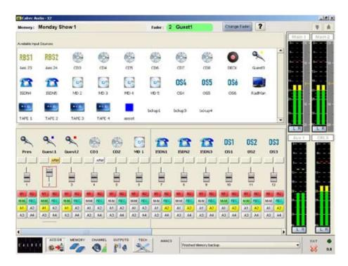
A red box around a screen fader indicates that the fader is open.
