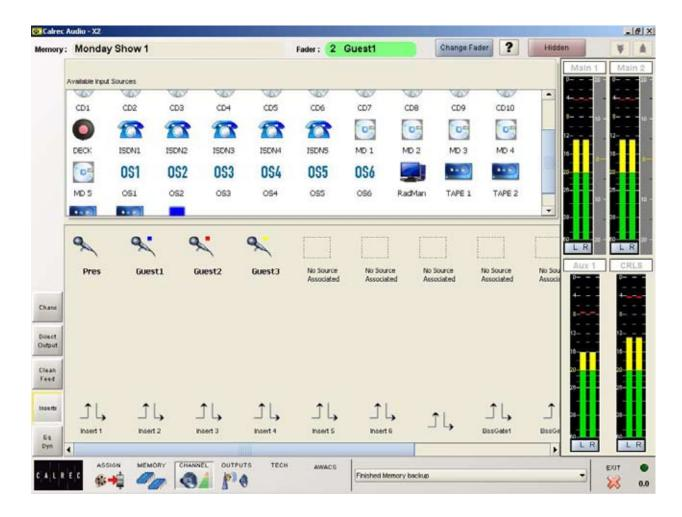
The system can have up to 48 inserts. Each insert can be allocated for use to one source using this screen.
