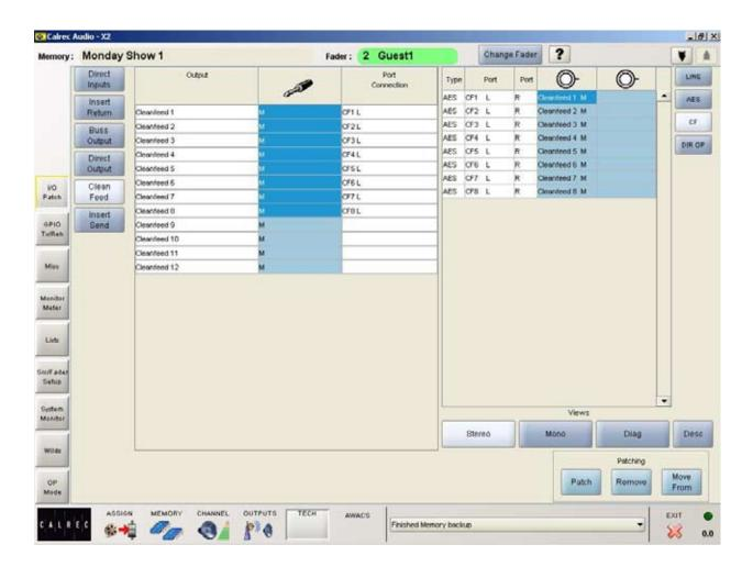
The Tech - I/O Patch - Clean Feed screen allows patching of clean feed outputs to output ports. This screen is only visible in engineer mode.
