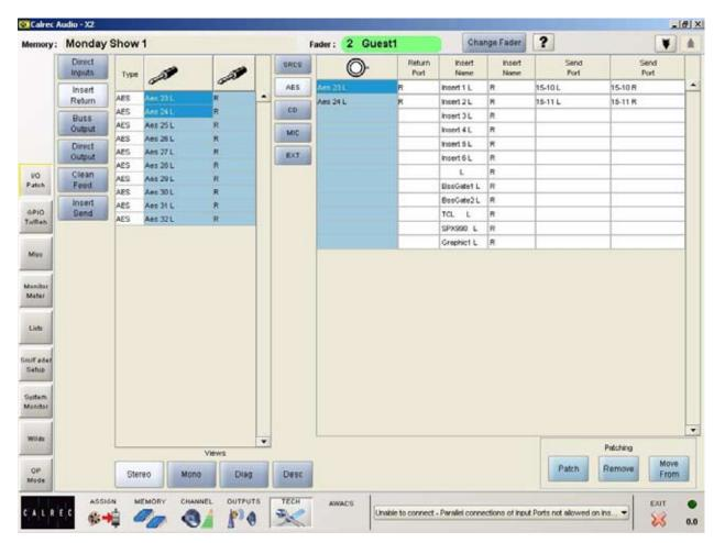
The Tech - I/O Patch - Insert Return screen allows patching of input ports to insert return signals. This screen is only visible in engineer mode.
