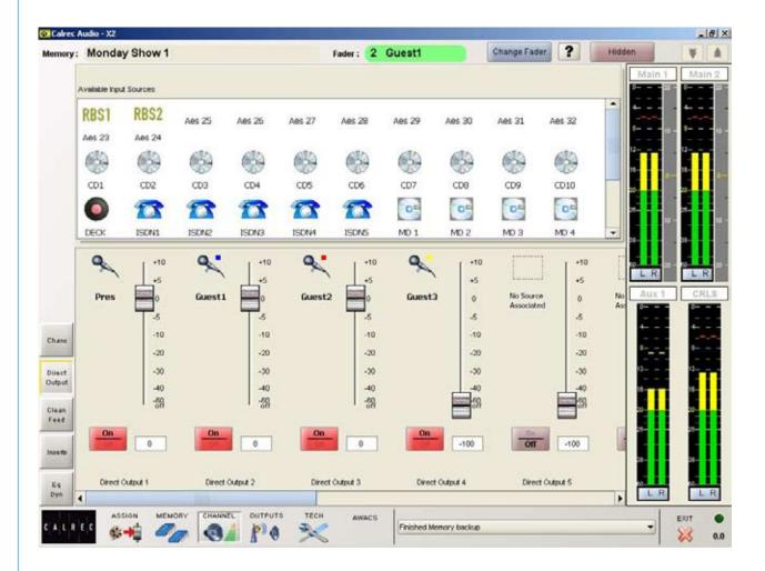
The system can have up to 30 direct outputs. Any input source can be designated as a direct output source.
