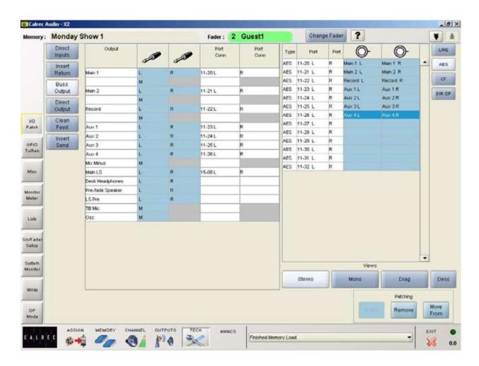
The Tech - I/O Patch - Buss Output screen allows patching of console output signals to output ports for mains 1 and 2, record, auxiliary, mix minus, monitor, talkback and oscillator outputs. This screen is only visible in engineer mode.
