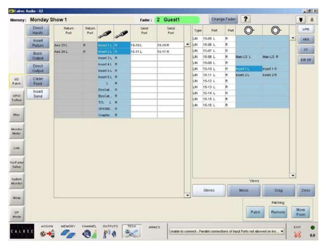
The Tech - I/O Patch - Insert Send screen allows patching of insert send signals to output ports. This screen is only visible in engineer mode.
