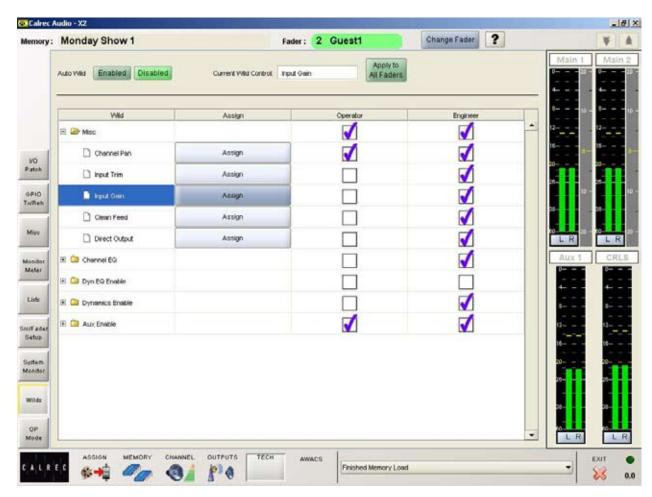
This screen allows the user to allocate functions to the faders' wild controls, and for studio engineer to restrict access to certain screens when in Operator mode.
