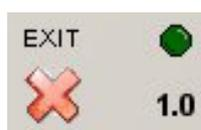
The "EXIT" button at the bottom corner of the screen will exit the application. Next to this button is an indicator which shows the status of the control processor. During normal operation, this indicator will be green. When busy, the processor's indicator will be yellow, during which time, no changes can be made to the control screens (Although changes to the control panels can be made, and will take immediate effect).
