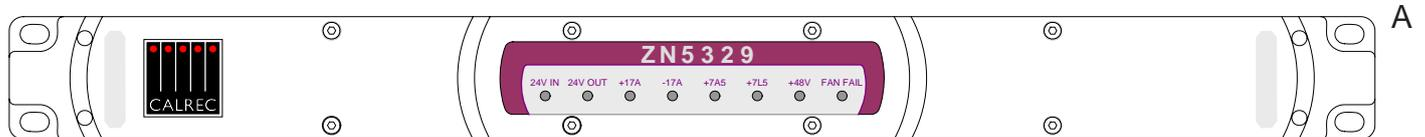
typical system would have two of these multi-rail power supply units, a primary unit powering the analogue components of the system, and the other as a “hot spare” providing redundancy, in case the primary unit fails. These units are monitored via the bulk power supply and distribution unit. Should a fault occur, the hot spare would automatically take over from the primary unit, the PSU Fail Indicator would begin to flash and a message would be sent to the control surface via AWACS.
