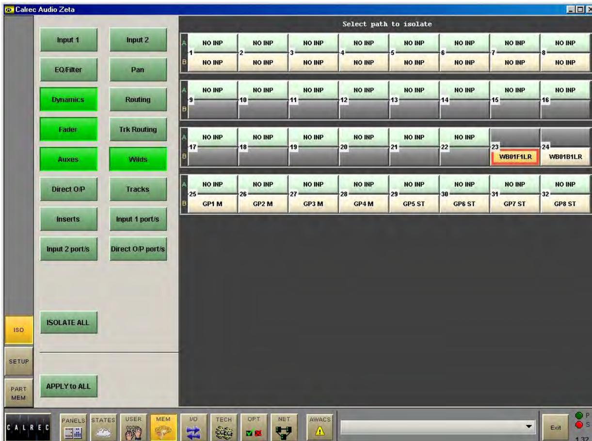
The Isolate screen allows some channel and group settings to be isolated from memory recall. This means their current settings will not be over-written when a different memory is loaded.
