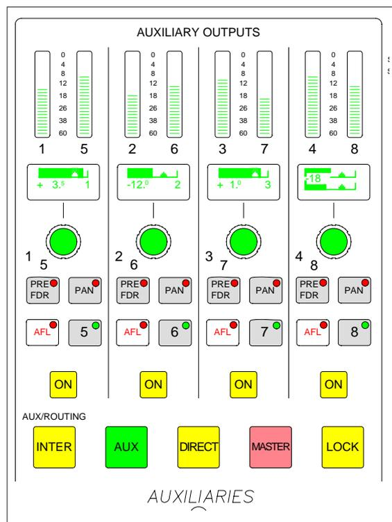
**INTER** This latching button puts the console into Interrogate mode. If the Aux ON buttons are held down, the fader assign buttons of all the paths feeding that buss will remain lit. The fader assign buttons of paths which are not feeding the buss will cease to be lit. It is also possible for interrogation of the routing busses to take place by holding down any of the routing buttons (groups, mains, tracks).
