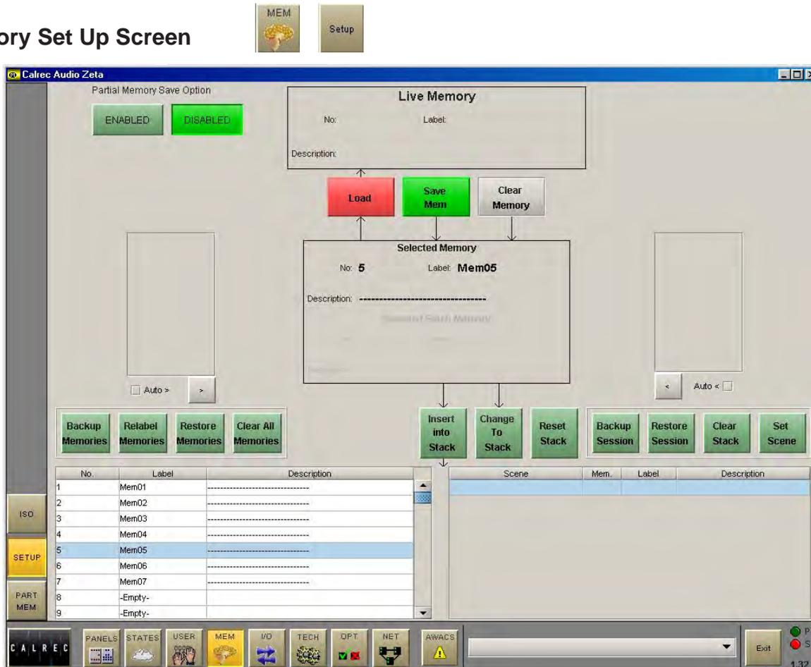
The Memory Setup screen duplicates the memory functions available on the control surface, and allows management of stored memories and stacks.
