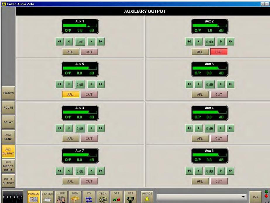
All of the auxiliary controls available on the control surface are available on the screens.
