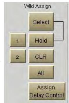
Wild controls provide the same function for paths A and B. The colour of the Wild control display indicates the path being currently controlled: Green for A, Amber for B. If the fader is touched instead of pushing a rotary control, then the fader for the alternate layer will be assigned to the Wild control.
