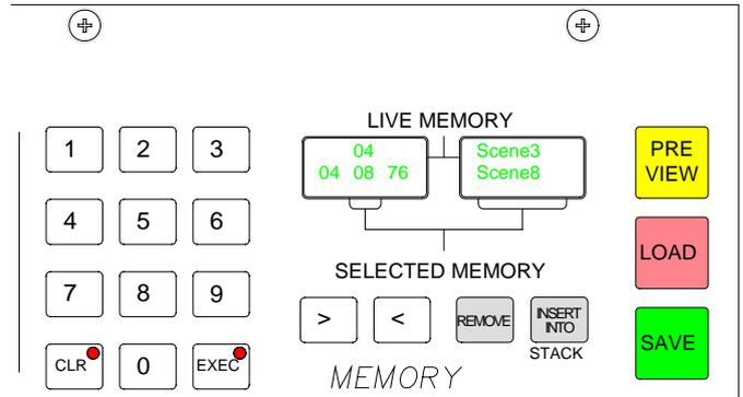
The buttons on this panel will affect the Selected Memory. The Selected Memory can be thought of as the “Ready” position, where the next required memory can be placed until it is needed.
