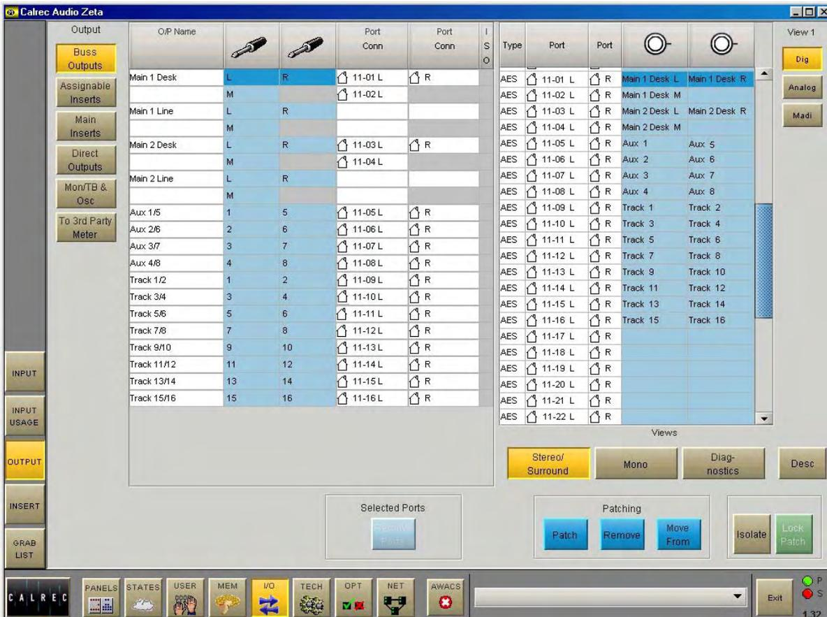
The right side of the screen shows the available output ports, which may have been grouped into lists during installation. Different lists are accessed using the selection buttons. The Output View buttons select the different categories of console output signals which can be patched to output ports. They will be displayed on the left section of this screen.
