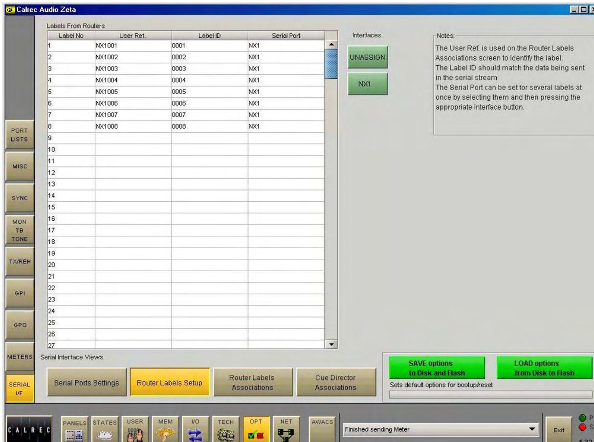
The serial port function previously set up on the Serial Port Settings screen will now have a selection button on this screen. To associate labels to the interface, select the label, or region of labels, and select the serial port function button. The serial port column tells the user which serial port function the label is linked to. The UNASSIGN button when selected will remove any assignment from the selected label(s).
