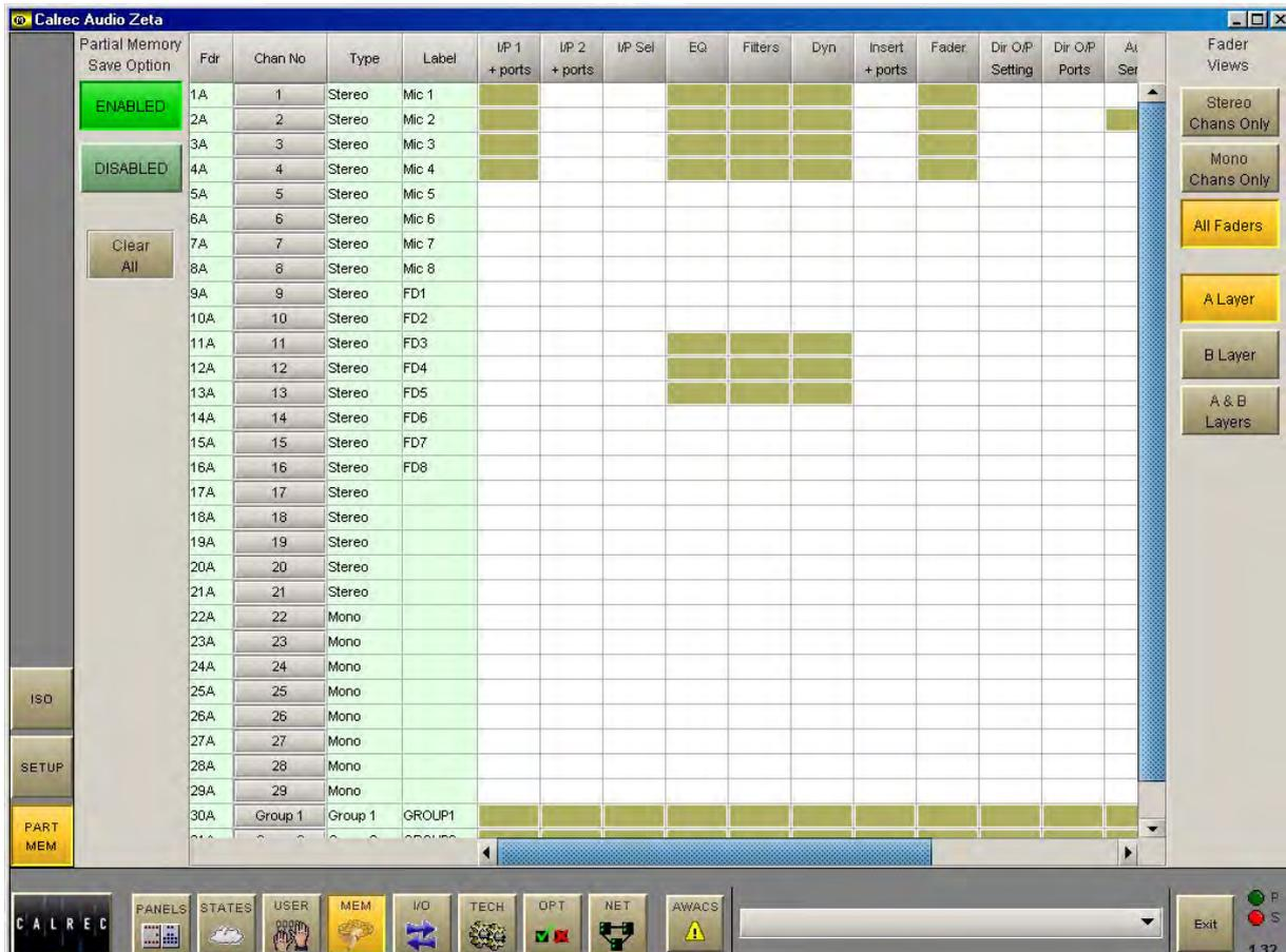
The Partial Memories function allows components of console settings to be saved in the same way as full console memories. When a partial memory is recalled, only the settings saved will be updated. The partial memories screen provides a mechanism for selecting channels or sub-components of channels to be saved in a partial memory.
