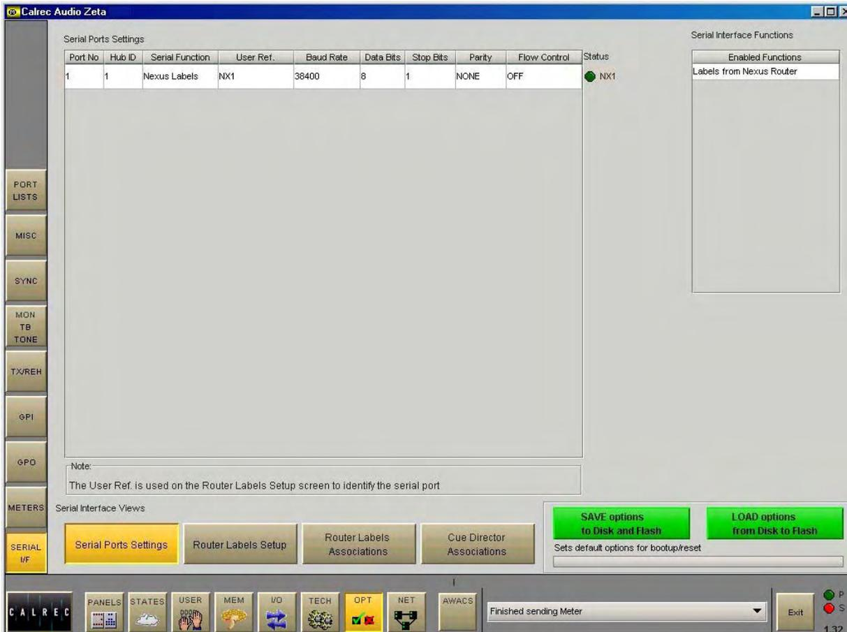
The console has a serial interface port for allowing equipment to be connected to the system. The Serial Port Settings screen is used to tell the system what information it should receive from the serial interface port, by allocating a function to it from a drop down box in the Serial Function column. Only the serial functions which are enabled for the console will be available for selection.
