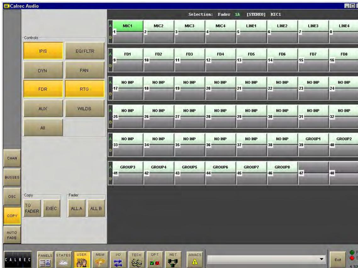
Eight sections of a channel or ALL together can be copied to another channel or channels using the User-Copy screen. First select the fader path you wish to copy, by pressing its fader assign button.
