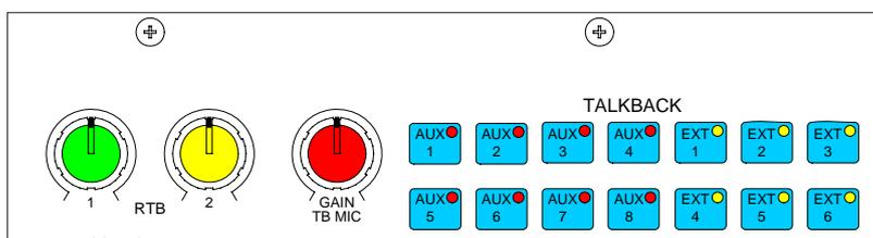
Talkback is available using the buttons in the track output section to individual tracks.
