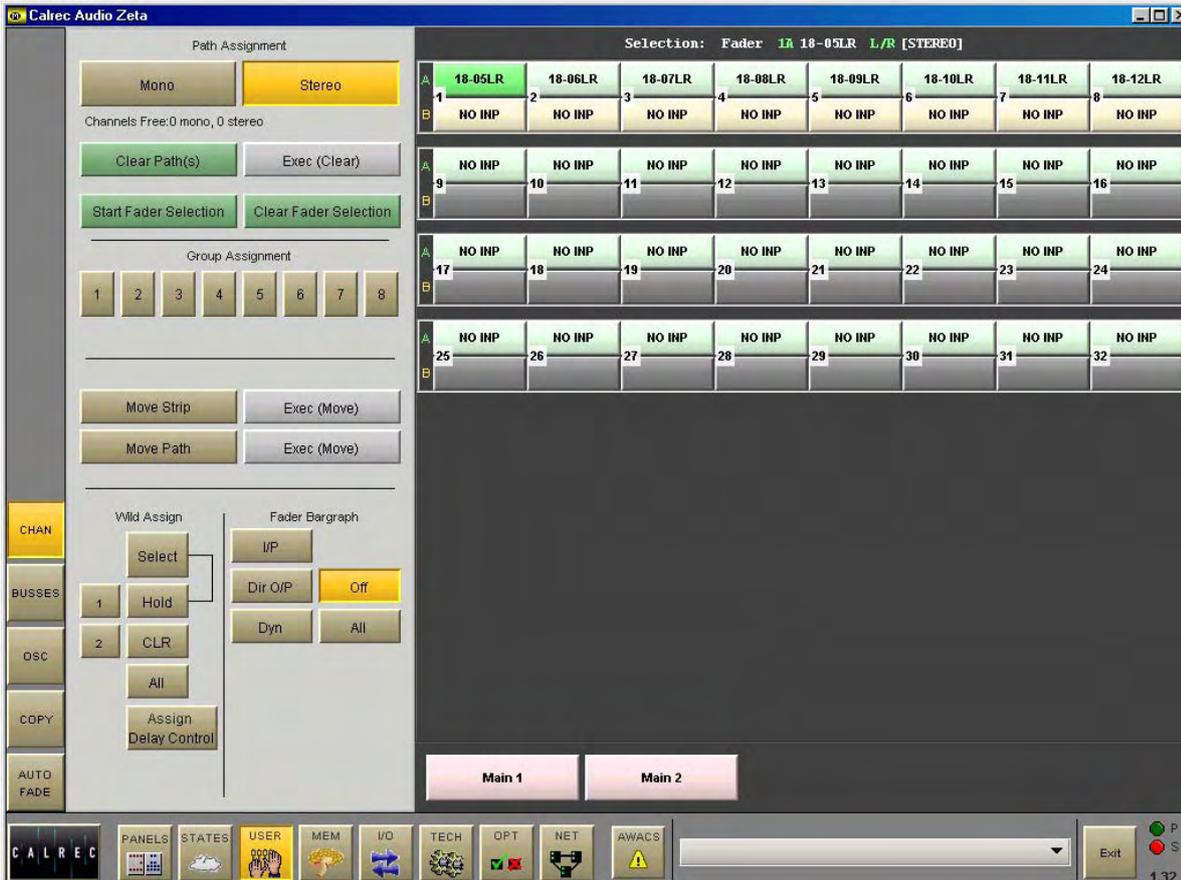
The right side of the screen shows the faders with buttons for paths A and B. To make changes, select the required fader either from the screen or by pushing its fader assign button. Then use the controls on the left side of the screen.
