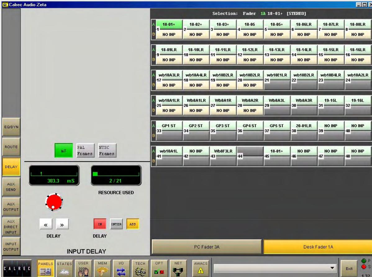
The Panels - Delay screen allows specific amounts of input delay to be applied to the currently assigned channel path. Alternatively, the user can choose to control a different fader, known as the “PC Fader”, to which delay settings can be applied independently of the current assignment. Control is chosen using the selection buttons.
