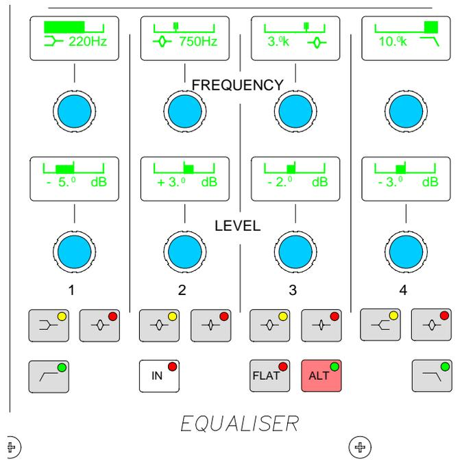
EQ level controls are adjustable by +/-15dB and are switched in and out of the signal path using the IN button. Bands overlap to allow greater flexibility of settings.
