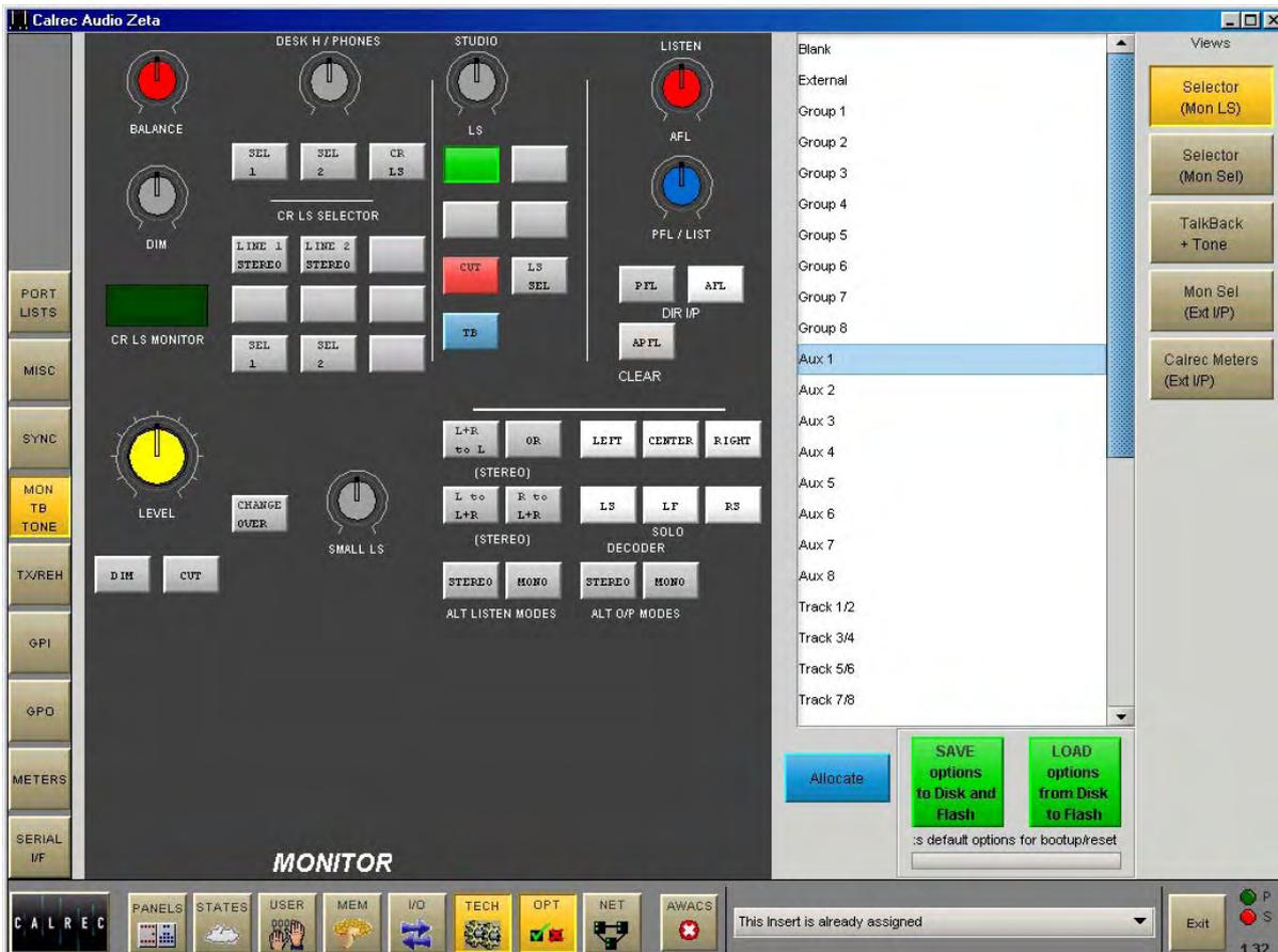
The screen allows the monitor LS user-definable buttons to be set up. The left side of the screen shows a representation of the monitor LS controls. The right side of the screen lists all the available monitor sources.
