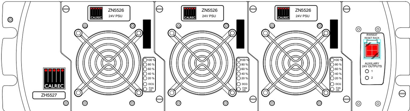
This 3U rack can hold up to 3 identical plug-in power supply units. Each unit has separate AC power inputs and DC outputs on the rear of the rack. Any one PSU can be removed from the rack without disturbing the operation of the others. A typical system would have one of these racks with 2 plug-in power supply units, one to provide power to the console control surface and digital components in the processing rack and another to act as a “hot spare”.
