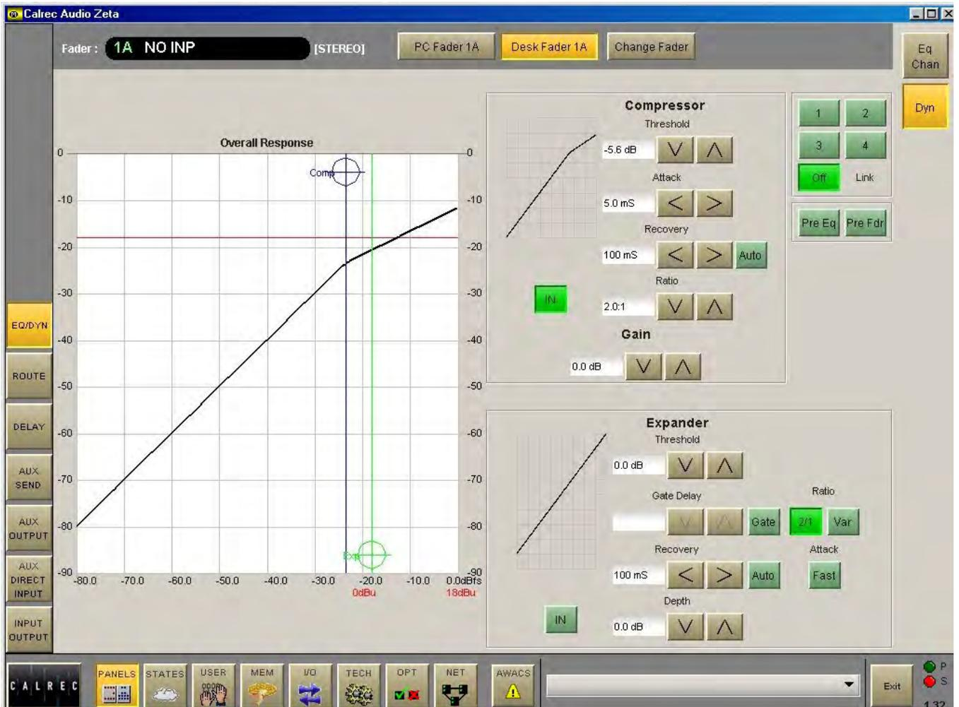
Compression or expansion settings can be adjusted using the touch screen, or trackball, by selecting the required crosshair and moving it around within the editable area. As it moves, the values will change. Nudge buttons to the right of the editable response window can also be used to make adjustments.
