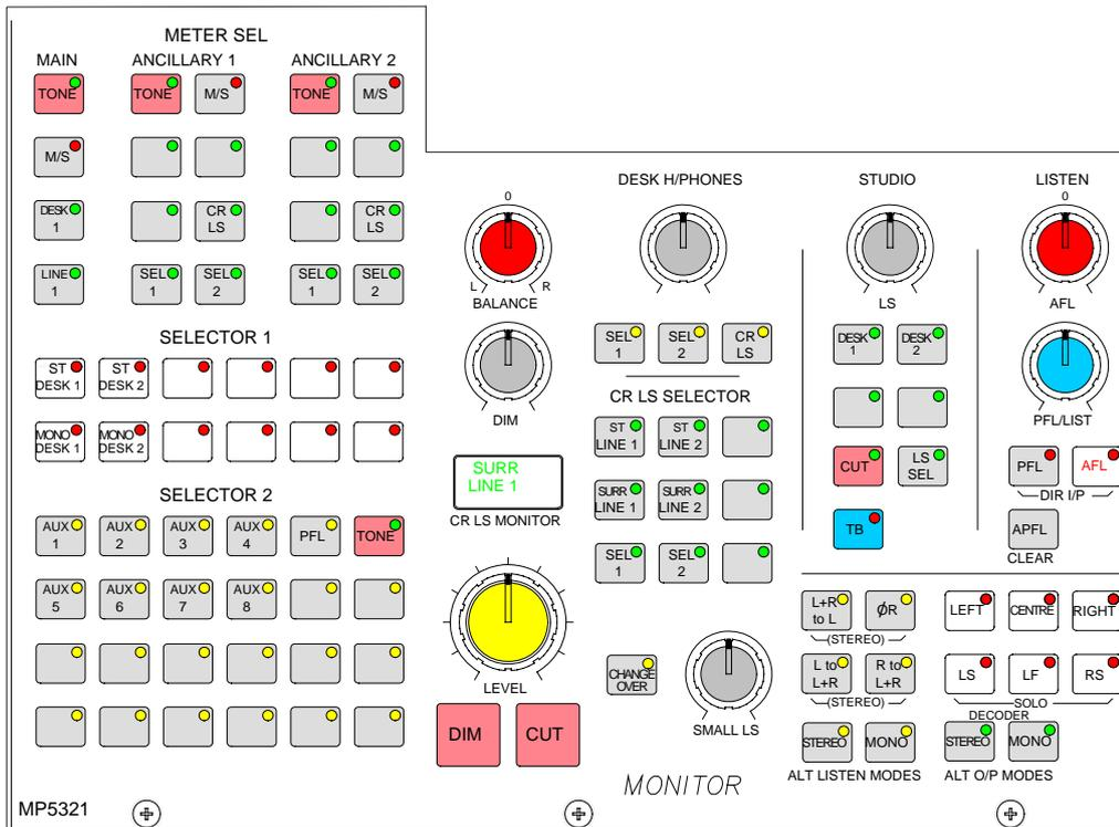
The Monitor Selector is used to select the source to monitor and the Meter Selector is used to select what to display on the meters. If the loudspeaker system is surround, stereo and mono sources will still be heard in stereo and mono, with no signals on the other speakers. Selector 1 and Selector 2 are sub-selectors which feed the other selectors. All selector external inputs can be mono, stereo or 5.1. Mono inputs are fed to L and R.
