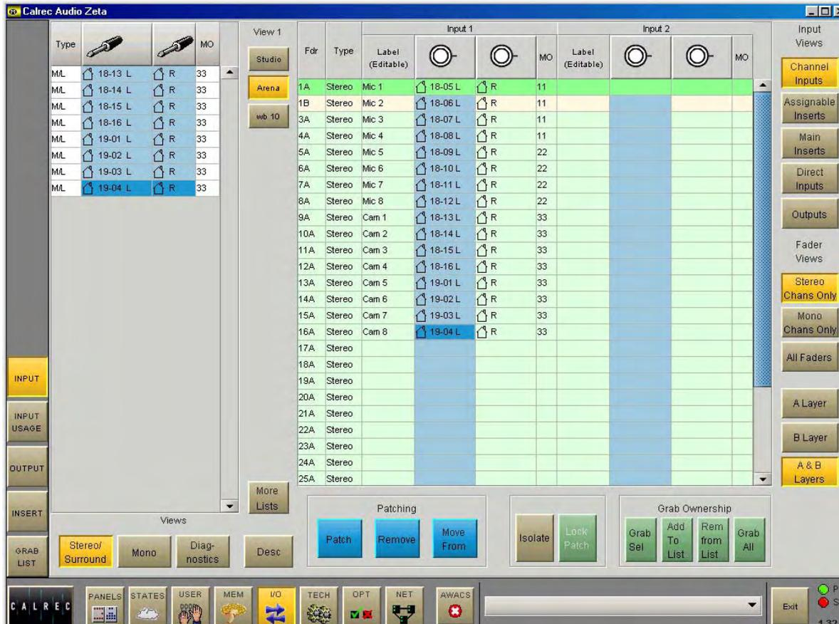
The left side of the screen lists the available input sources, which may be grouped into lists. Different lists are accessed using the selection buttons. The Input View buttons on the right side of the screen select the different console input functions which can have input ports attached. They will then be displayed in the main section of this screen.
