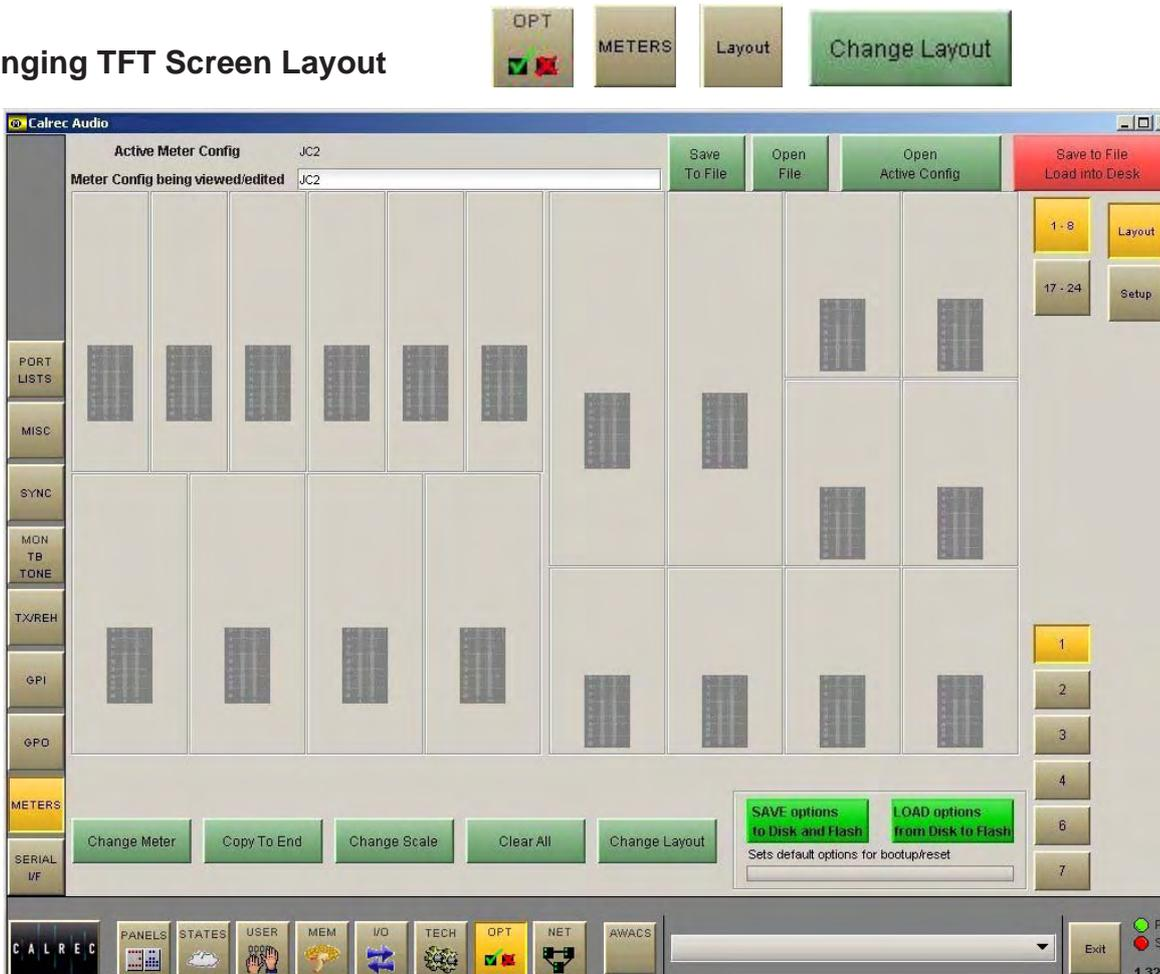
The user can control the layout of the rows and columns on the TFT screens. The numbered buttons allow the meter in that upstand position to be selected for set up.
