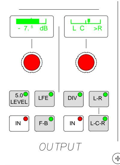
Divergence sets an amount of the centre signal to also feed to the left and right. Divergence does not operate on stereo channels and groups.
