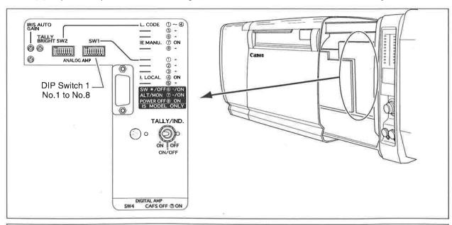
※ (NOTE): DIP switch 1 No. 8 is the IS main off switch.
