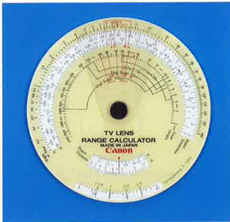
Fig.26 Canon Range Calculator for TV lenses
