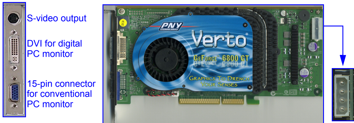
Figure 8-7. GeForce 6800 GT card. Left: Signal connectors. Right: Internal power connector.
