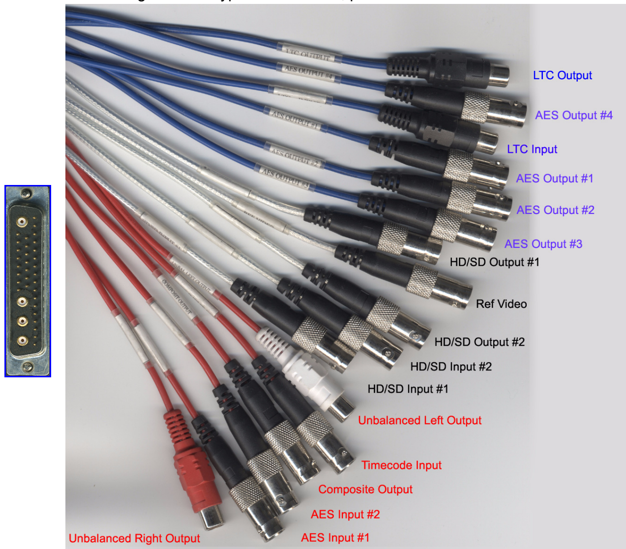
Figure 4-5. HyperX eFX Board breakout cable; compound connector at left
