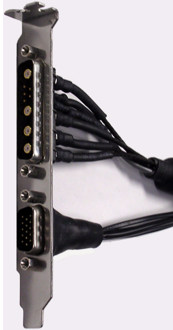
Figure 3-12. DigiSuite LE digital video (top) and audio connectors.
