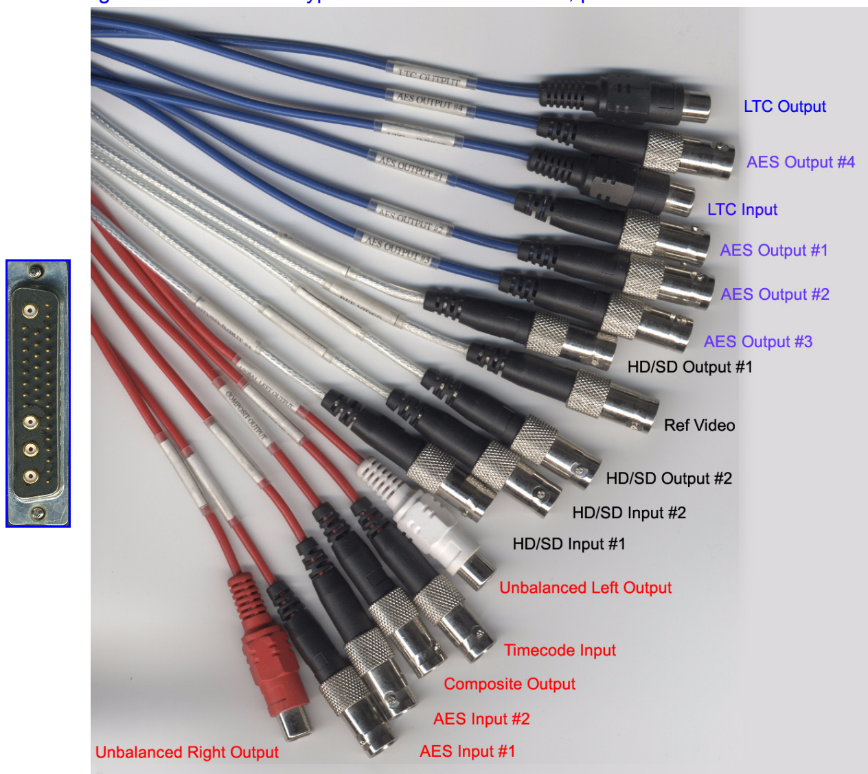
Figure 3-10. "Altitude" breakout cable; compound connector at left
