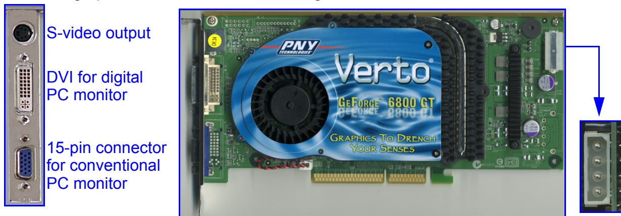
Figure 6-8. GeForce 6800 GT card. Left: Signal connectors. Right: Internal power connector.
