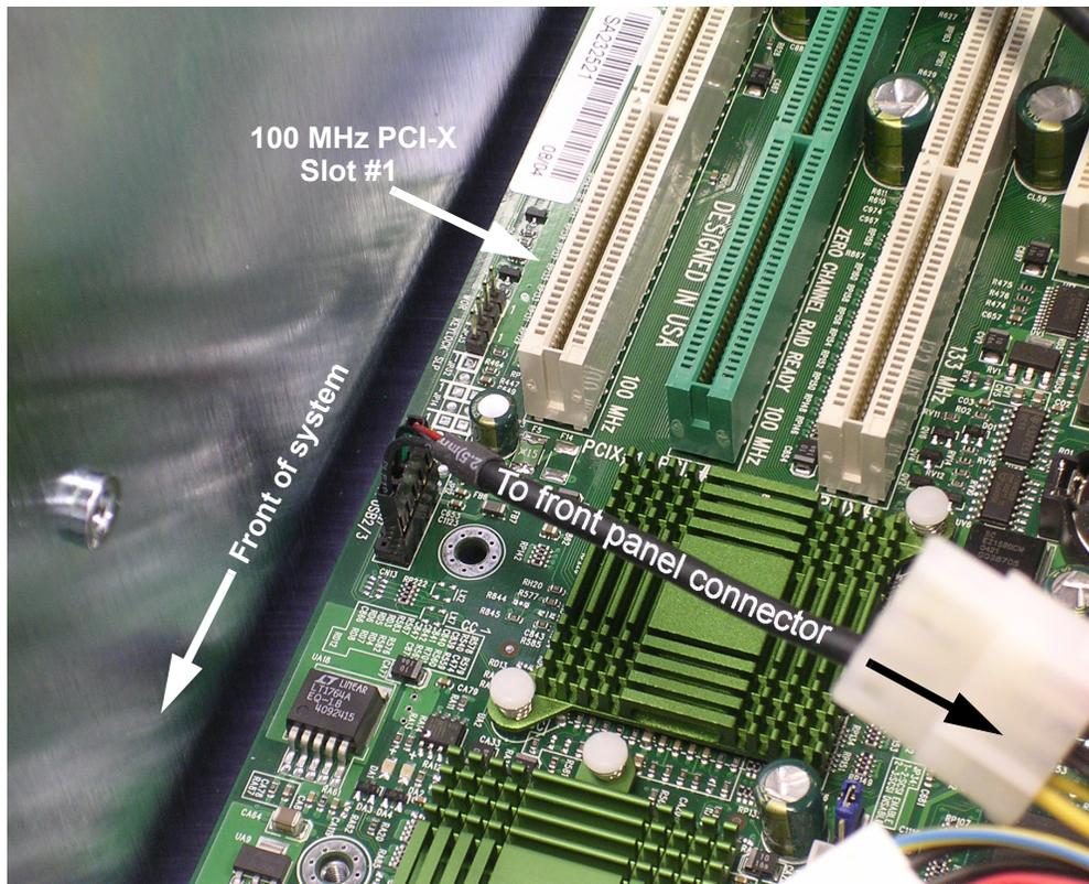
Figure 8-4. Close-up view of motherboard's USB connector
