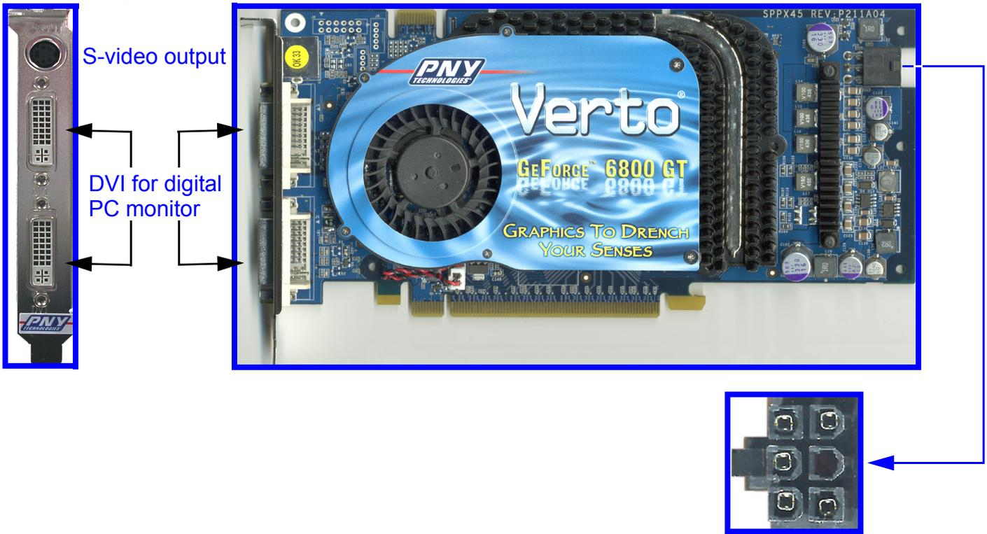
Figure 7-7. GeForce 6800 GT card. Left: Signal connectors.
