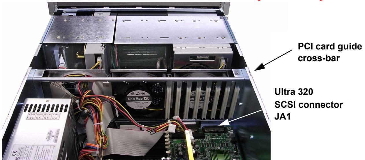
Figure 6-2. HyperX interior, showing rear of disk drives, SCSI connector
