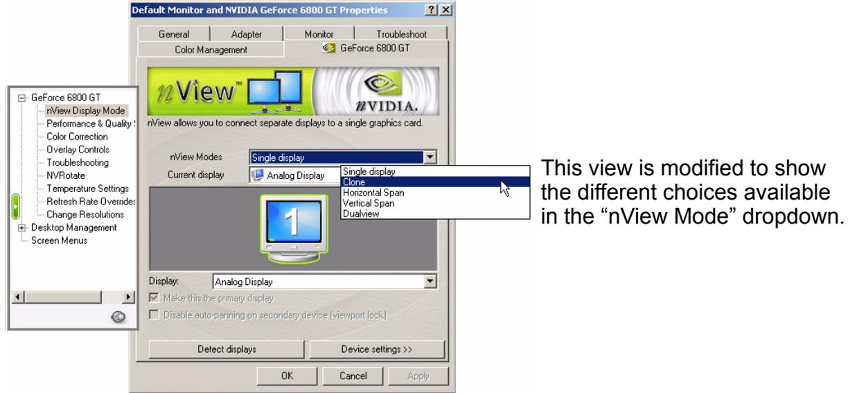
Figure 5-5. Option for “cloning” VGA display on TV monitor
