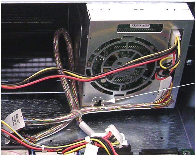
Power connector to side fan, located directly behind SCSI drive bays
