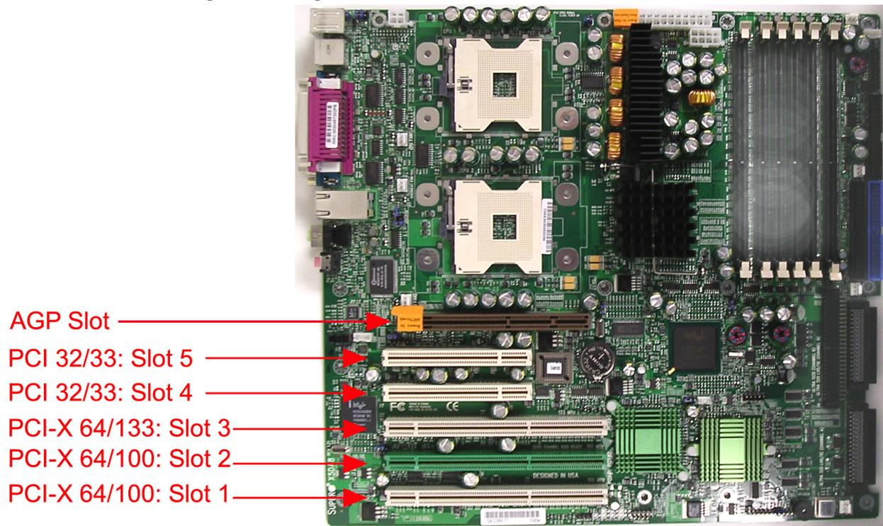
Figure 8-8. PCI and PCI-X slots, numbered at right
