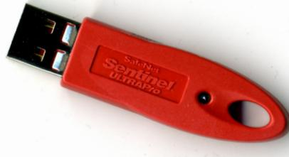
Figure 6-4. “Dongle” USB security device.
