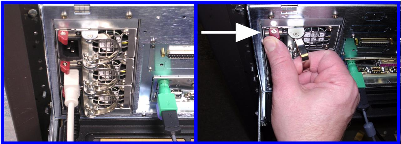
Figure 6-8. Replacing a power supply module
