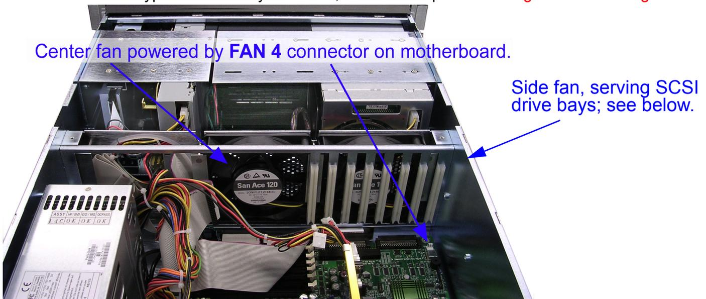
Figure 6-12. Power connection to center system fan
