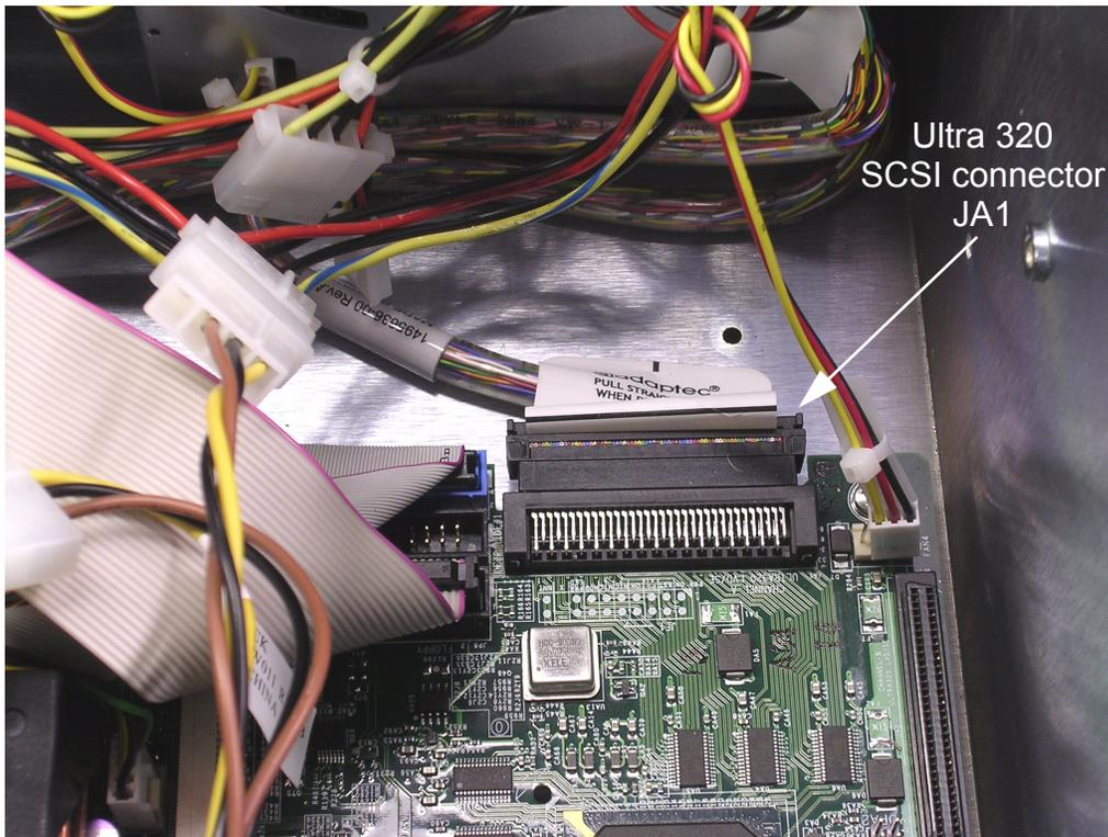
Figure 6-6. Close-up of SCSI connector JA1.
