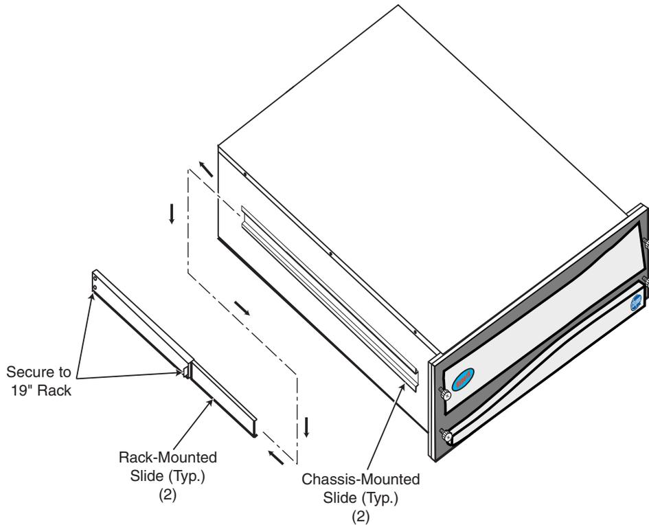
Figure 3-1. Duet HyperX and its rack-mounting hardware
