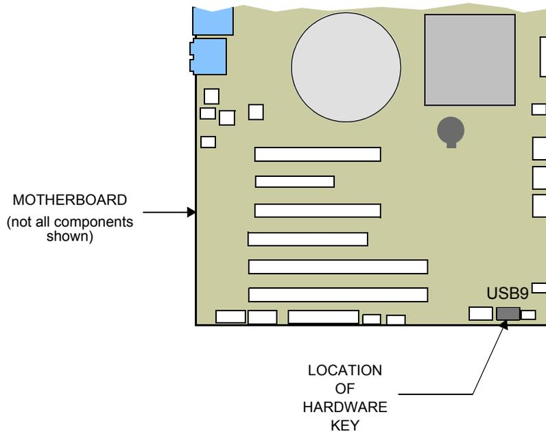
**Figure 8 USB Hardware Key**
