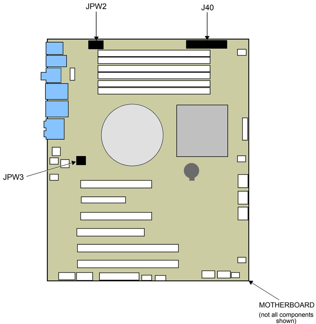
**Figure 12 ATX Power Connections**
