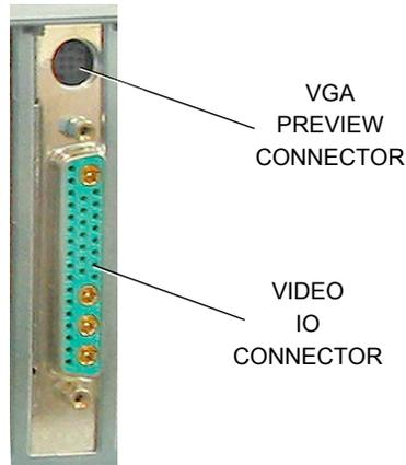
**Figure 7 eFX Board Connectors**
