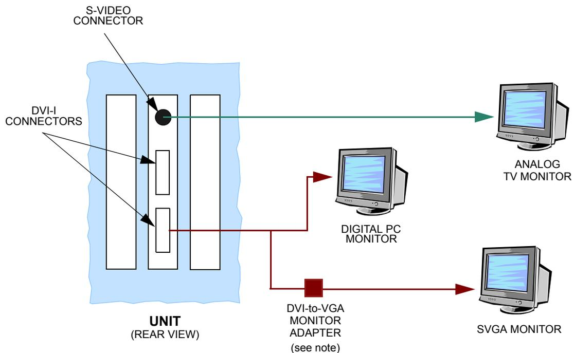
**NOTE:** two DVI-to-VGA monitor adapters are provided--one for each DVI-I connector.
