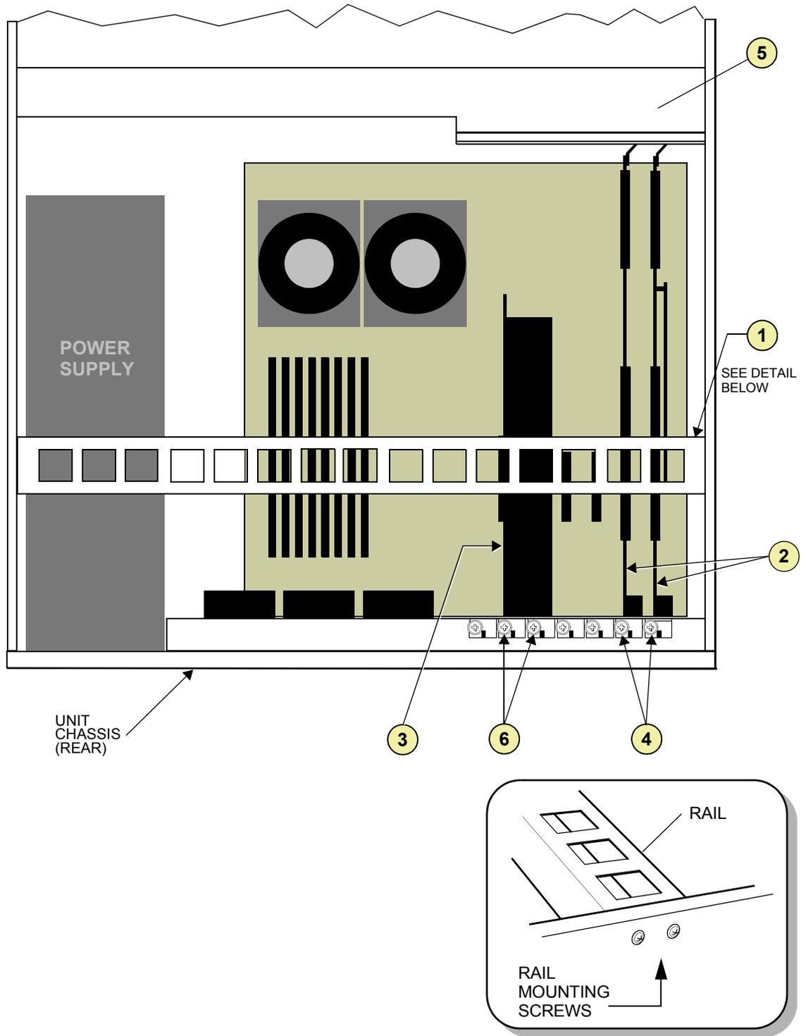
**Figure 16 Removal/Replacement of Circuit Boards**
