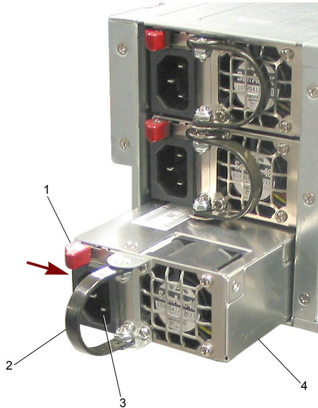
**Figure 13 Power Supply—Hot Swap Procedure**
