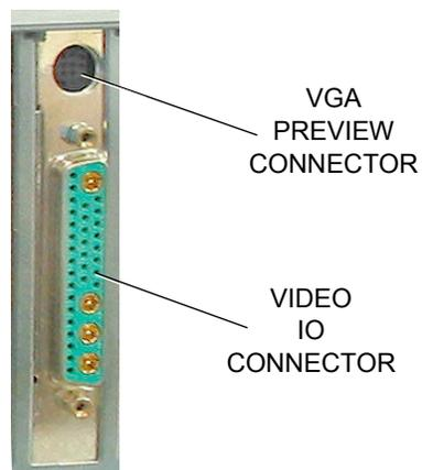
**Figure 5 eFX Board Connectors**
