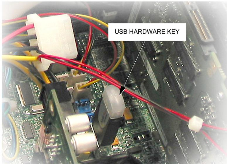
**Figure 8 USB Hardware Key**
