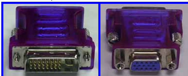
Figure 5-9. The included DVI-to-VGA monitor adapter
