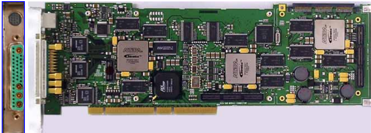
Figure 4-4. HyperX eFX Board; panel connector at left
