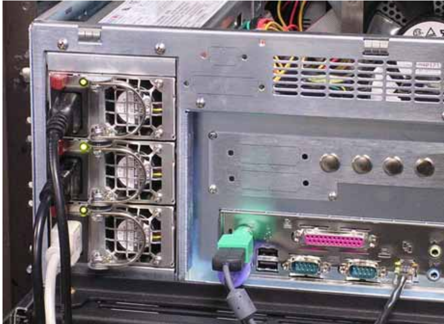
Figure 6-9. Indicator lights on each power supply module; other rear panel details may vary.
