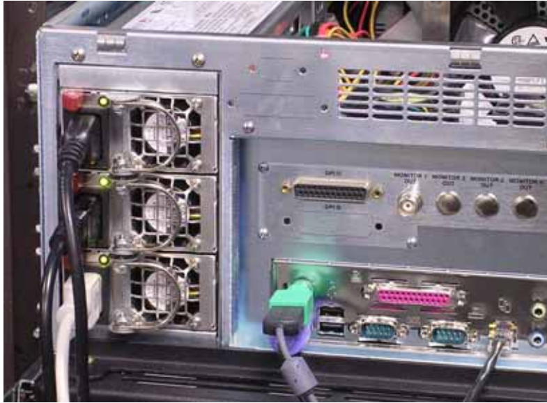
Figure 5-1. Stand-by LED indicators, left, show that the module is receiving power. Your system's appearance may differ from this illustration.
