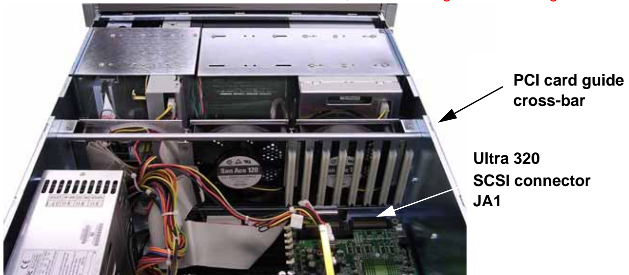
Figure 6-2. HyperX interior, showing rear of disk drives, SCSI connector
