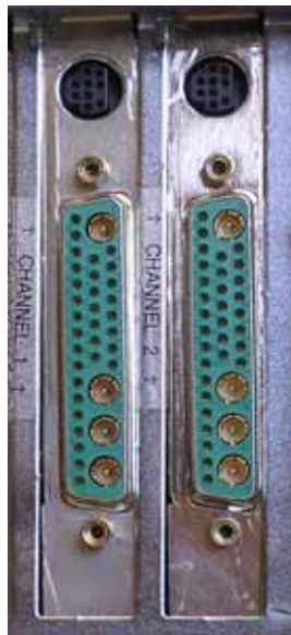
Figure 4-3. Frame Buffer numbers labelled on rear of a HyperX configured with two eFX Boards. Your system's factory configuration may differ from the one seen here.
