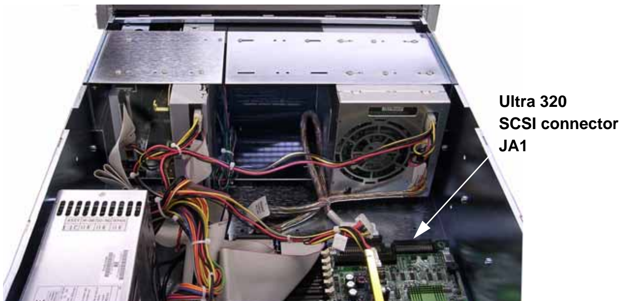
Figure 6-3. HyperX interior, PCI card guide cross-bar removed for visibility
