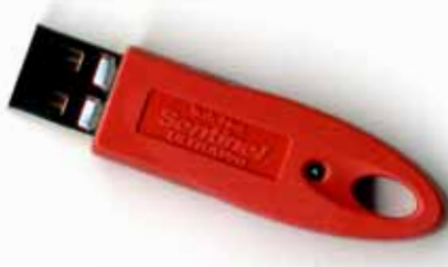
Figure 6-4. “Dongle” USB security device.
