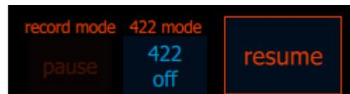
When "pause" is pressed, ingest is halted, the file remains in an open but static state and the record/pause button changes name to "resume".
