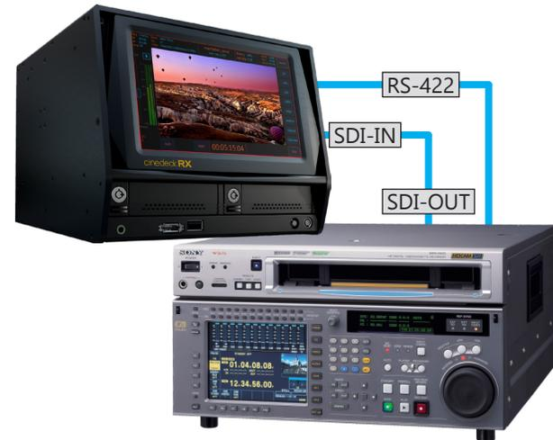
Whether working channel to channel or from a separate source machine to the Cinedeck, the operator can control the player channel / machine via RS-422, using the controls provided on the Cinedeck target channel interface.
