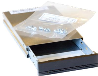
To install the SSDs, open the carrier and remove the screws.
