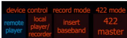
Insert Baseband mode allows the replacement of content in any selected region of many closed file types. The user can open a file on the Cinedeck, set an in and out point, along with the appropriate video and or audio channels which need replacing and trigger insert recording to fill in the selected area, with whatever is coming into the SDI input. Inserts can be video, audio, or audio with video.
