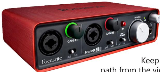
Lastly, a XLR or TRS balanced audio pair can be introduced to the system using a Focusrite 2i2 USB audio adapter.
