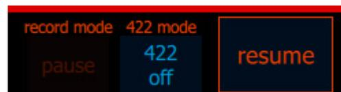
When in resume, the record (red border) indicator will blink on and off, indicating that record mode is still active but ingest has been paused.
