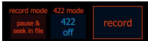
Pause & Seek in File is similar to “pause” mode but pause & seek in file also mimics the “assemble edit mode” commonly used on a tape machine. In “pause & seek”, when pause is pressed, ingest is halted and the file remains open like in standard “pause” mode. Then the recently recorded
