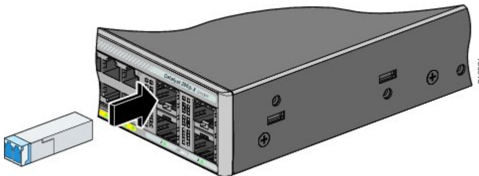
Figure 30: Installing an SFP Module
