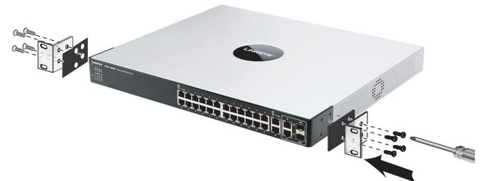
3. Place a rack mount bracket next to the spacer and reinstall the four screws (removed in step 1).
