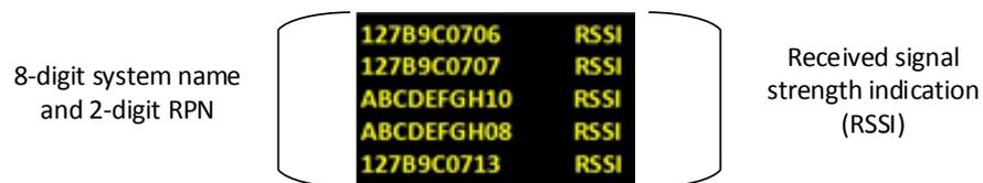
**Figure 3-4 An unconnected beltpack site survey screen**
