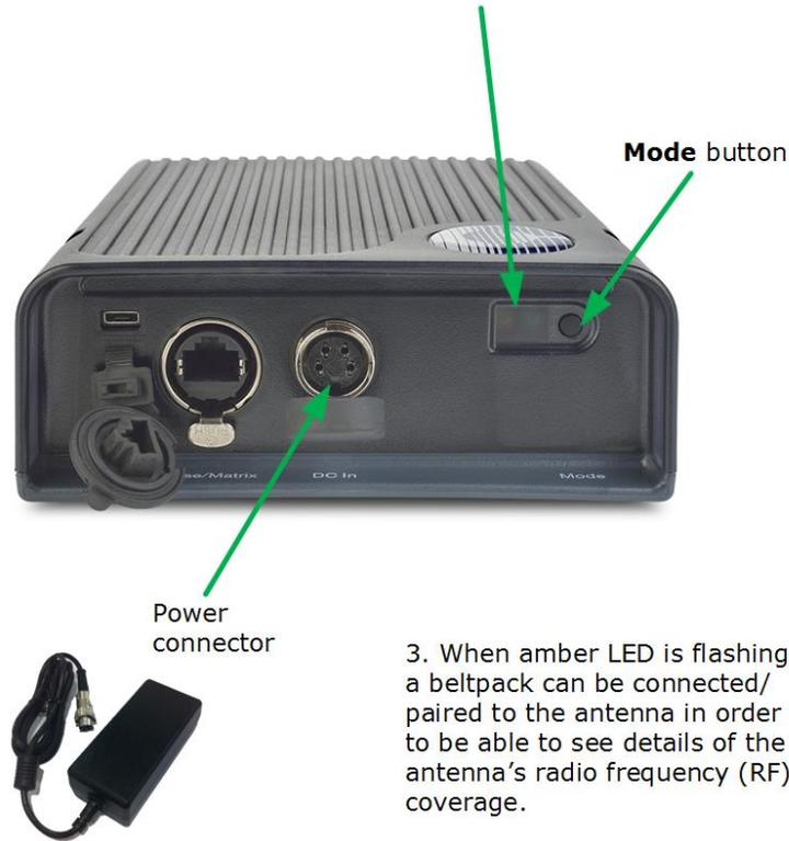
3. When amber LED is flashing, a beltpack can be connected/ paired to the antenna in order to be able to see details of the antenna's radio frequency (RF) coverage.
