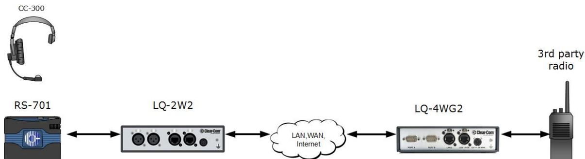
This example shows how to send a GPO (General Purpose Output) trigger to a third party radio when audio comes in from an Encore RS701 beltpack. This can be used to open audio transmission on the radio; equivalent to pressing the Push To Talk (PTT) button on the radio.
