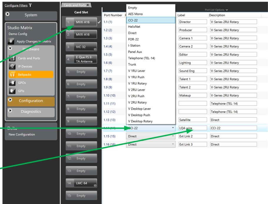
**Note:** The connection between the MVX or PiCo and the LQ device is a 4-wire connection, even though it is declared as a 2-wire connection.
