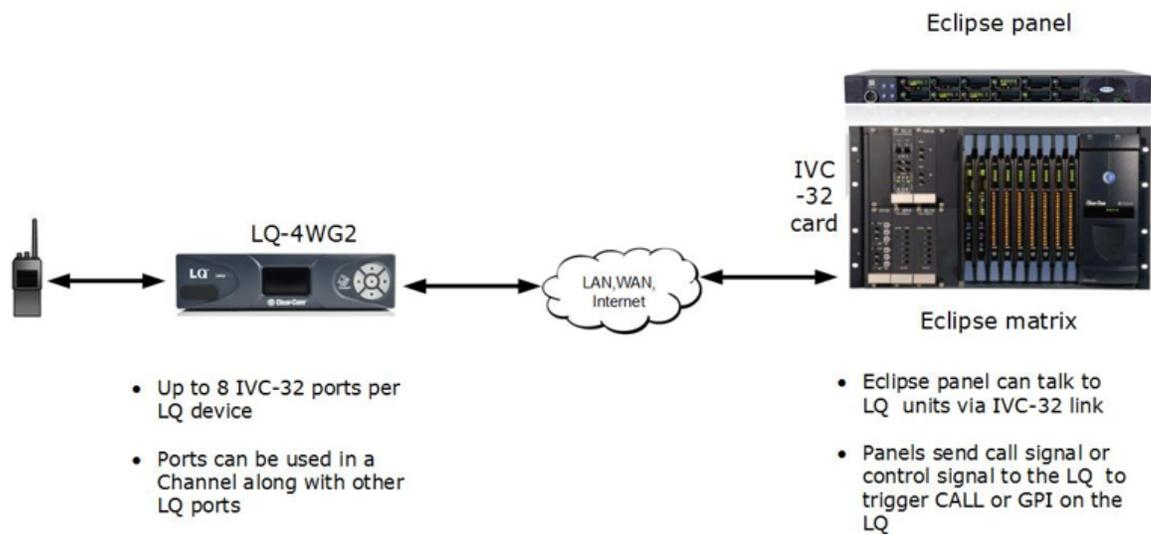
Each LQ-R unit supports up to 24 ports: 8 hardware ports, 8 SIP ports and 8 virtual ports. Agent-IC and IVC ports are considered 'virtual' ports. Virtual ports can be used in any combination up to 8 in total.
