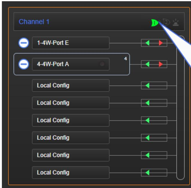
When audio triggers the VOX on Port E, Port A will fire a GPO. The **Network Control Event** icon lights when this happens.
