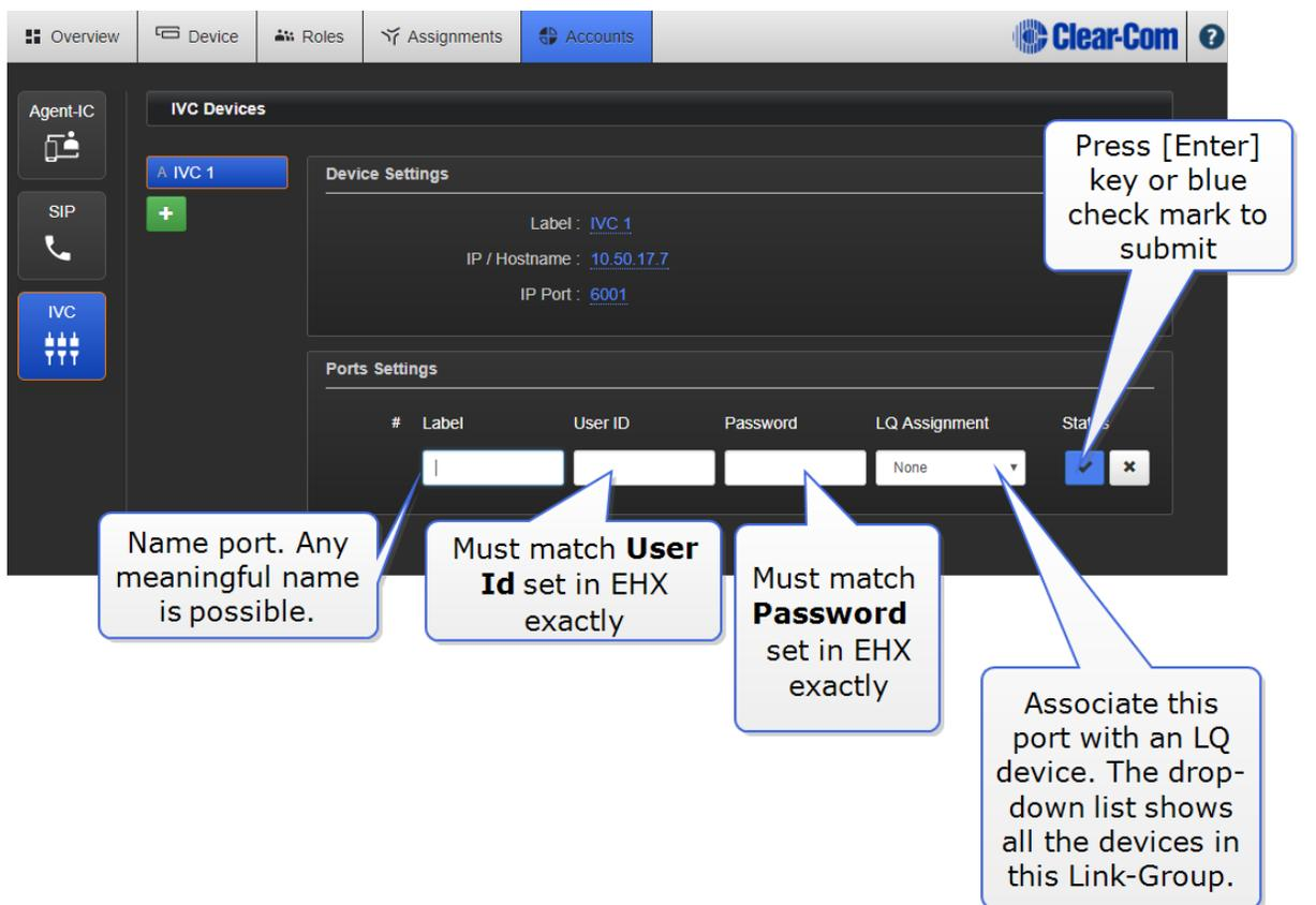
When the LQ is connected to the IVC-32 card, a green status LED shows. If the connection is not successful, a yellow warning displays. Click the yellow warning symbol for information.
