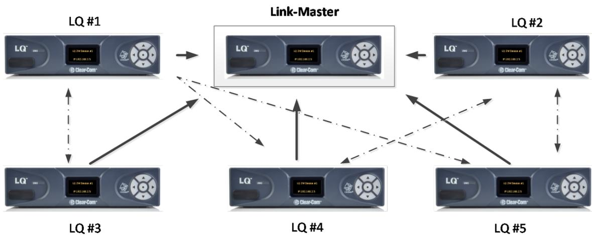
LQ units establish a robust mesh network when transporting audio (see image above). The units use a series of IP ports to create this mesh:
