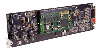
The 9323 is a HD/SD embedder/de-embedder with sample rate conversion, audio level, channel phase inversion, channel mapping and video level controls.
