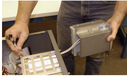
Figure 5-29: Inserting DVD/CD Floppy housing assembly back into workstation
