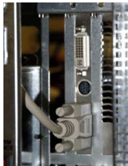
Figure 5-8: Monitor cable connected to SVGA card.
