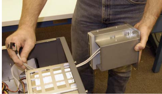
Figure 5-27: Removal of DVD/CD and Floppy Drive
