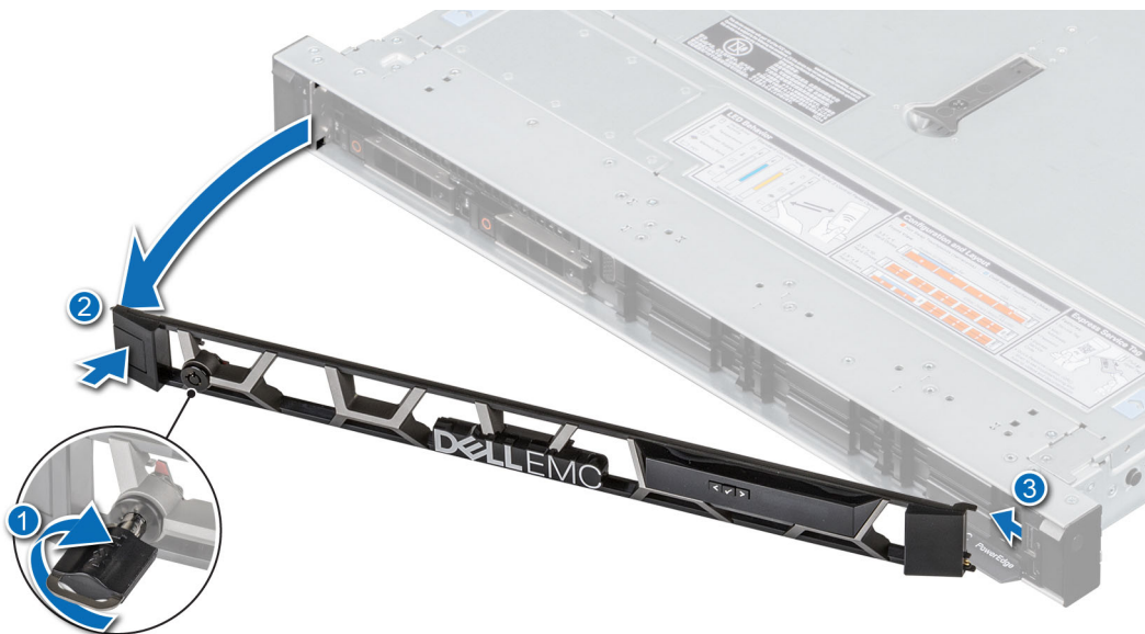
Figure 15. Removing the front bezel
