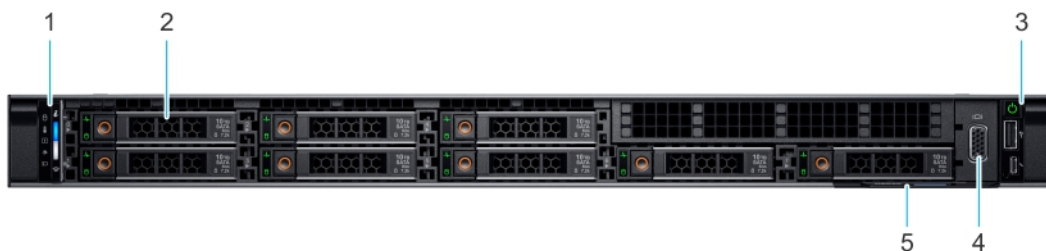
Figure 2. Front view of the 8 x 2.5-inch drive system
