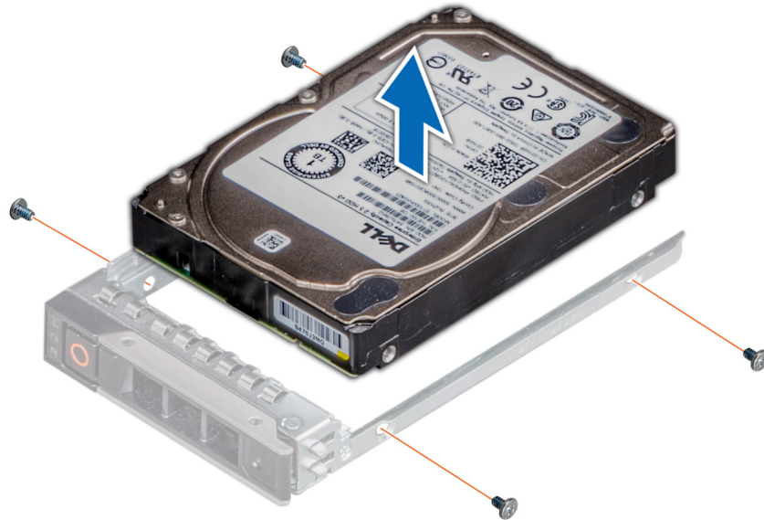
Figure 37. Removing the drive from the drive carrier
