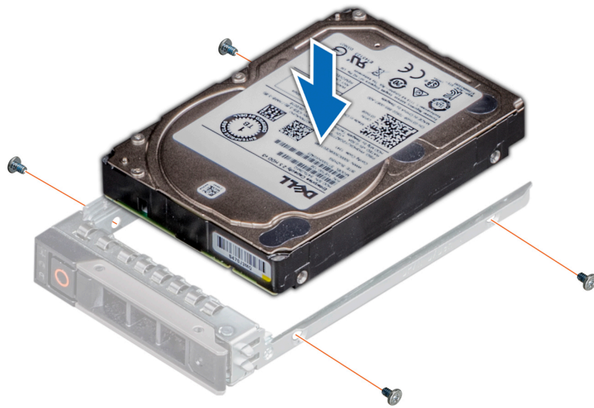
Figure 38. Installing a drive into the drive carrier
