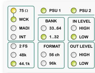
Clock source is 'word clock' with termination enabled. Conversion of channels 01-32.
