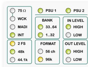
Clock source is set to internal clock generator. Conversion of channels 01-32 (i.e. all channels)\*.
