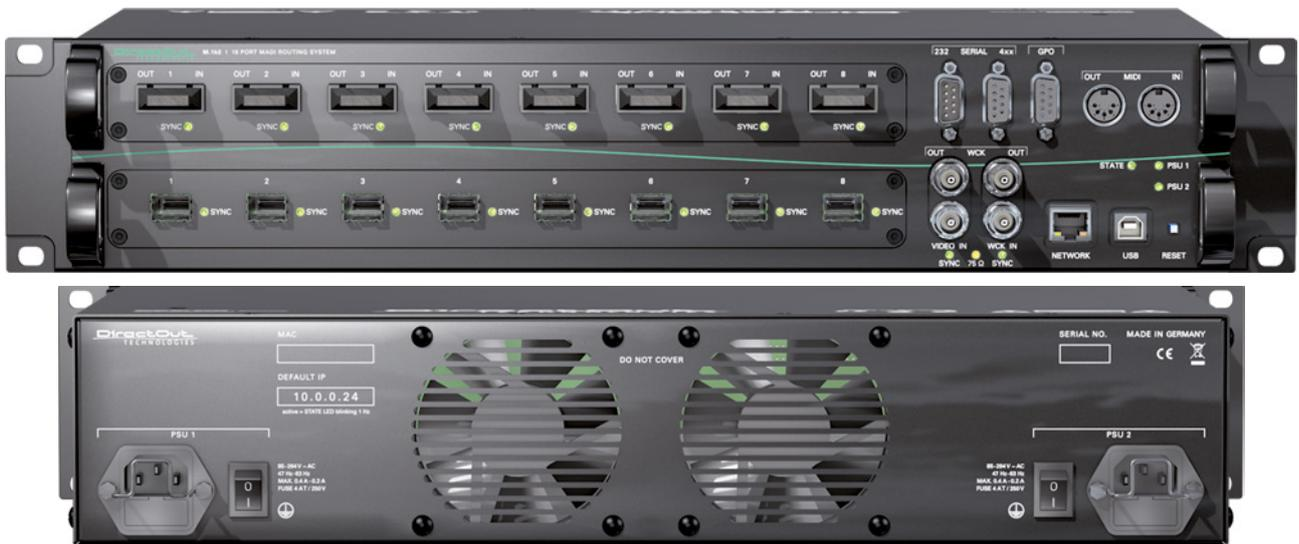
You can distribute MADi signals en bloc in a port matrix and you may also create your own MADi stream using the channel matrix. PolySync™ provides the ability to use different clock sources on individual ports. So the router may be divided into single 'clock groups' that can run at different sample rates.
