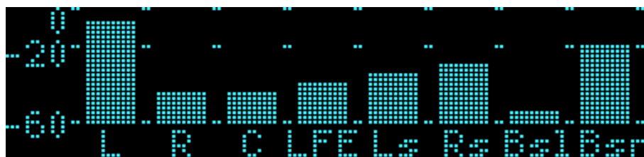
Figure 4-8 Level Meter Displaying a Dolby E 7.1 Input
