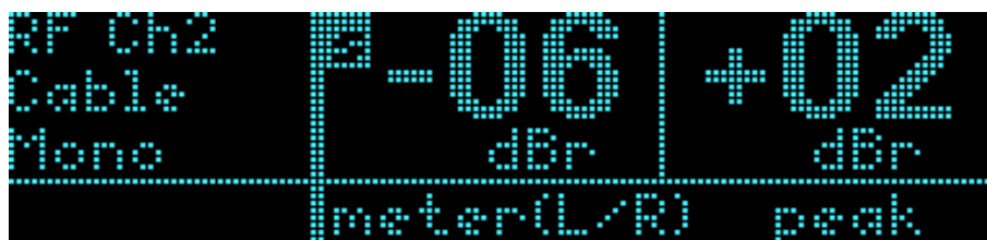
Figure 4-6 Main Status Screen when Receiving an RF Signal
