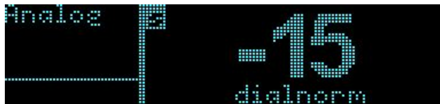
Figure 4-7 Main Status Screen Displaying a Recommended Dialnorm Setting for an Analog Input
