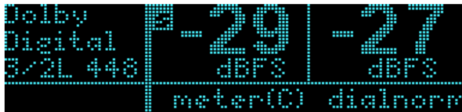
Figure 4-1 Main Status Screen when Receiving a Dolby Digital Stream
