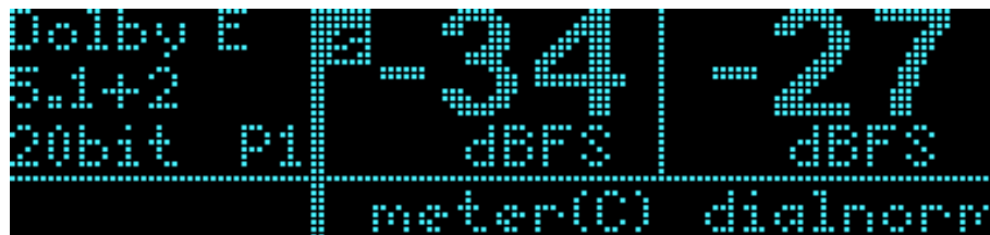
Figure 4-3 Main Status Screen when Receiving a Dolby E Stream
