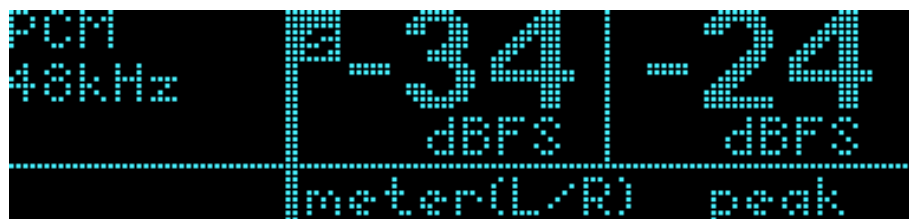
Figure 4-4 Main Status Screen when Receiving a PCM Signal
