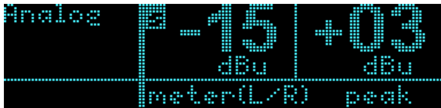
Figure 4-5 Main Status Screen when Receiving an Analog Signal
