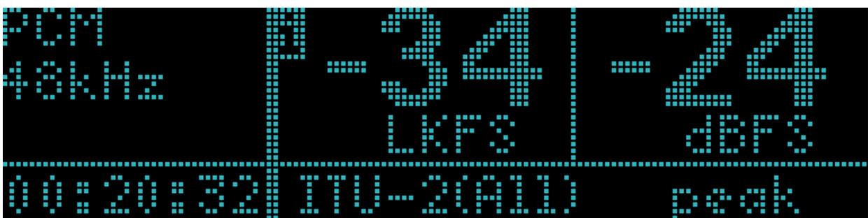
**Figure 4-7** Main Status Screen when Receiving a PCM Signal
