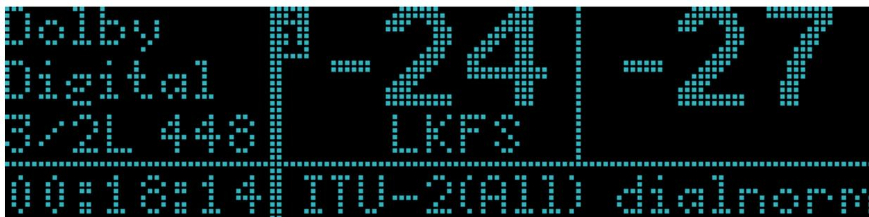
**Figure 2-3** Default Measurement Display Example
