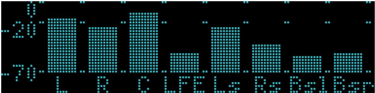
**Figure 4-11** Level Meter Displaying a Dolby E 7.1 Input
