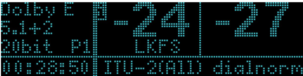
**Figure 4-6** Main Status Screen when Receiving a Dolby E Stream
