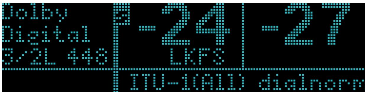
Figure 4-3 Main Status Screen with the ITU-R BS.1770-1 Measurement Type
