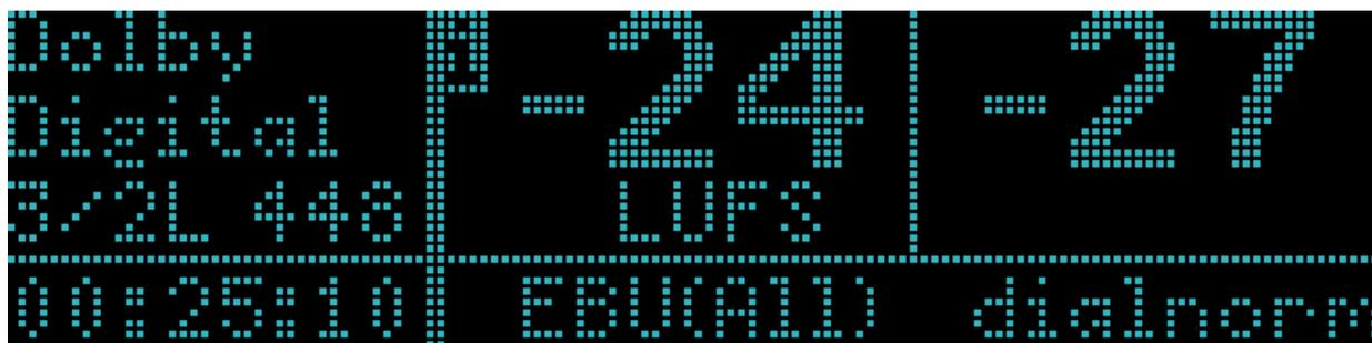
Figure 4-2 Main Status Screen with the EBU R128 Measurement Type
