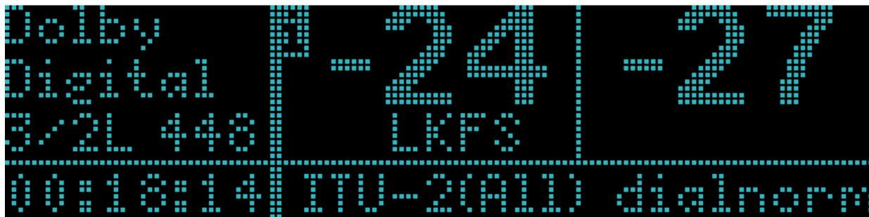
Figure 4-1 Main Status Screen with the Default ITU-R BS.1770-2 Measurement Type
