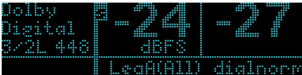
Figure 4-4 Main Status Screen with the Leq(A) Measurement Type
