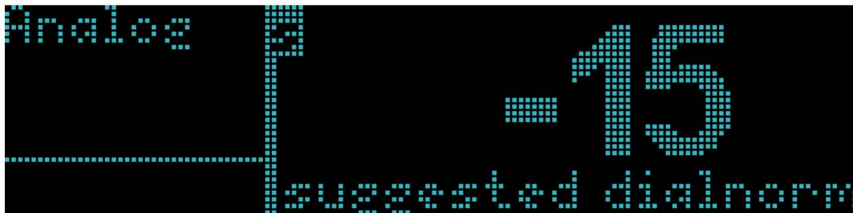
**Figure 4-10** Main Status Screen Displaying a Recommended dialnorm Setting for an Analog Input
