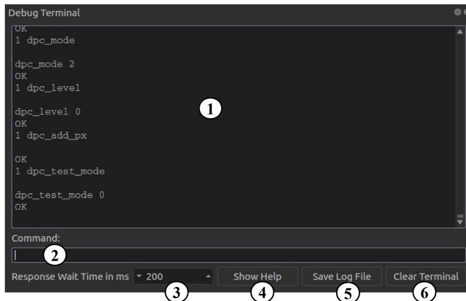
The Debug Terminal shows all commands which are sent by the GUI. It can also be used to manually send commands to the device.
