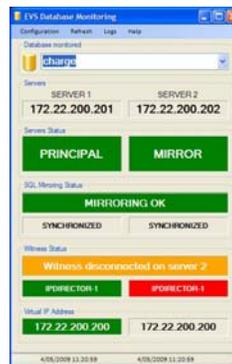
The “EVS Database Monitoring” monitors the EVSDBIP status on 2 database servers (typically the principal and mirror server). The application shows the status of the EVSDBIP service, the status of the mirroring, the witness information and the status of the EVSDBIP virtual IP address.
