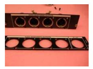
10. Modify the position of the power switch cables to place correctly the new rear panel.
