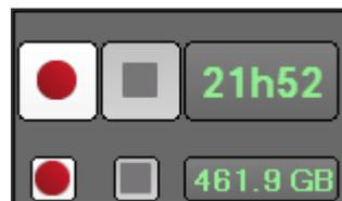
The remaining capacity on the EVS video servers is displayed in time.
