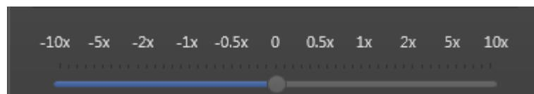
The slider can be dragged to the left or to the right to respectively play backward or forward. It returns to the zero state as soon as the mouse button is released.
