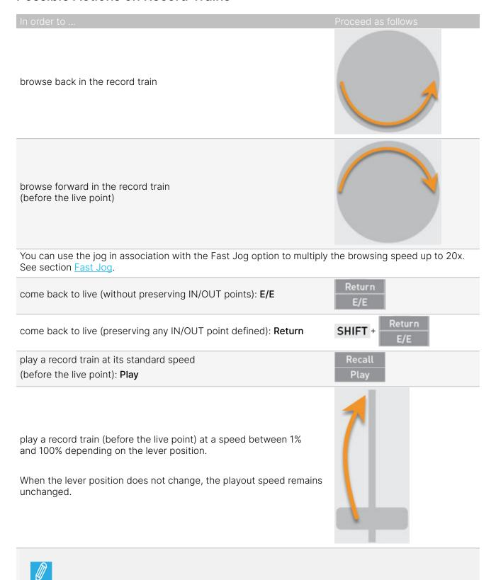
When supermotion material is loaded on the primary channel, the lever range has a larger, flat step at 50% in SLSM 2x, 33% in SLSM 3x, ...
