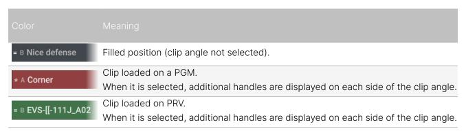
When a clip angle is selected, colored handles are added on each side of the clip position, whether the clip is loaded or not. The selection is blue for local clips and purple for remote clips. If the clip is not loaded, the whole clip position is colored as well. If it is loaded, the clip position will be colored as mentioned above.
