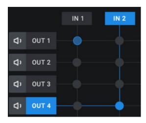
A **Mute** button is available next to each OUT track. When the track has been muted, the button turns orange as well as the intersection dot.
