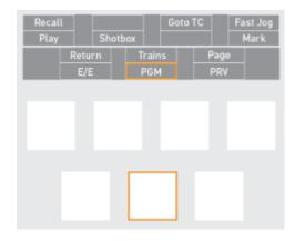
• When you are in PRV-only control, press the **PRV** key to take control on both PGM and PRV:
