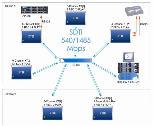
Only servers with HCTX board with SDTI module and SDTI code can be connected to the XNet network.
