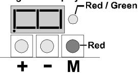
Green  $\rightarrow$  you must select the parameter you want to adjust. +/- buttons can be used to scroll through parameters.
