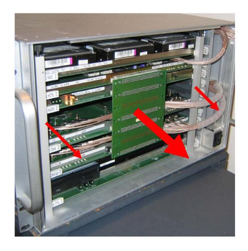
3. Unplug carefully the SMB connectors on COHX GLK (n°2) and COHX (n°4) boards.
