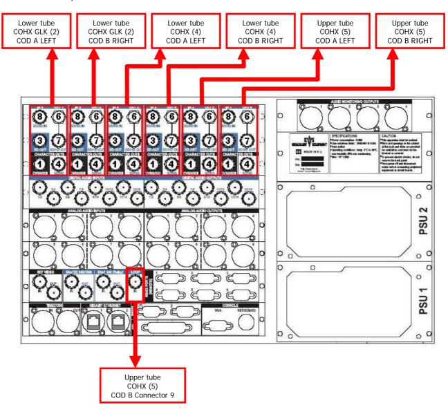
Important: Unplug the LOOP IN connector from COHX (4) COD B connector 9, slide the TEFLON cable off the lower tube and slide it into the upper tube. Finally connect it on the COHX (5) COB connector 9.
