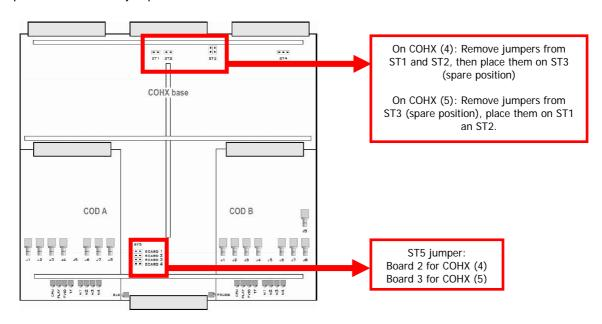
Jumpers ST1 and ST2 must be closed on the upper COHX board as a termination.
