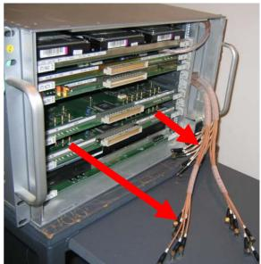
4. Remove the white "spirotubes" off the TEFLON cables.
