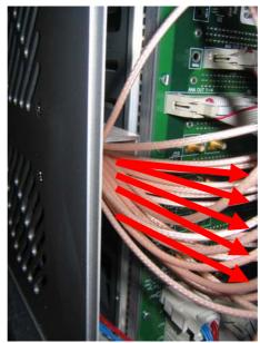
7. Exchange the 4 CH BNC back panel with the 6 CH BNC back panel.
