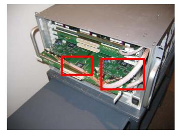
Plug the COD B connectors with the same method as described before and join cables together with white "spirotubes" (or tie-raps).
