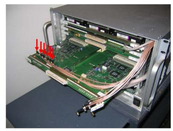
Plug first the COD A connectors regarding the numbers labelled on TEFLON cables. There is only 6 cables per channel (1,3,4,6,7&8). Please refer to the *point 8* picture to do it.
