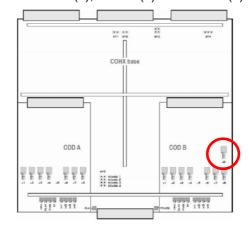
Warning: Don't forget the extra connector 9 on COHX (5) for the LOOP IN option.
