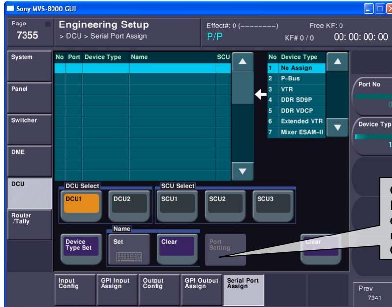
**Important:** To correctly recall the video to the Spotbox-XT PGM Outputs... you MUST define a valid PORT SETTING. This allows the MVS-8000 to indicate which video output the clip recall should be routed to. In Port Settings, the user changes from 0 to a number that matches the PGM output of the Spotbox-XT.
