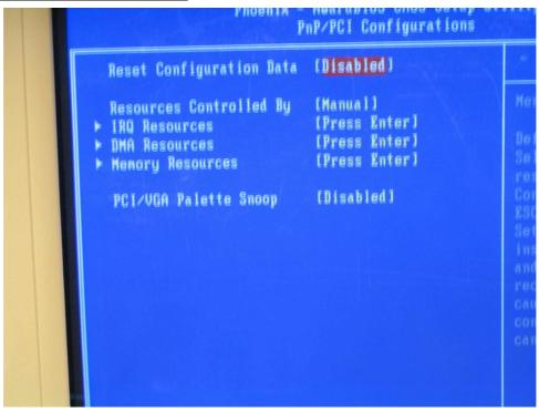
On this page select the line (with >) and press ENTER to have access on each sub-folder for configuration.
