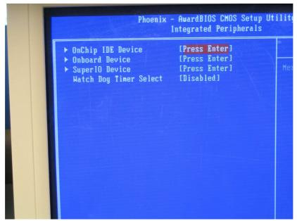
On this page select the line (with >) and press ENTER to have access on each sub-folder for configuration.
