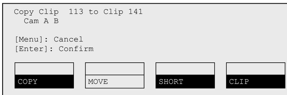
4. Select the **COPY** or **MOVE** function by pressing the **A** or **B** key.
