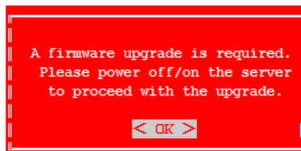
The message ask you to power off/on the server. A simple reboot of the software is not enough, **you have to turn off/on the power switch**. During the restart, the quad MTPC will be upgrade. Once the upgrade finished, the server continue to boot normally. The total duration of the operation (upgrade Multicam + quad MTPC and restart) is around 12 minutes.
