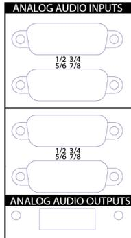
The analog audio inputs and outputs are available on 4 multi-pin DA-15 connectors with (2 in and 2 out) for audio signal inputs and outputs in analog format.
