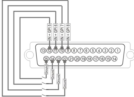
The relay must be connected between the ground and the corresponding TTL input on the DB-25.
