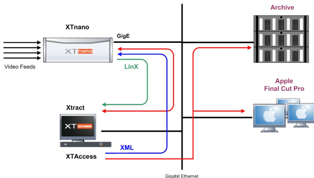
XT Access is directly connected to the XTnano servers through the Gigabit network. It runs on an XP workstation and is controlled, in this context, by Xtract via XML files.
