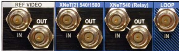
Loop mode is now possible on an XT[2] Server, however it can not be performed internally and requires a physical connection (BNC to BNC cable) between the BNC socket marked LOOP on the back plane and an output from the channel to be replayed (the LOOP connector overrides the connection to input 1 of the XT when the LOOP function is enabled on the remote panel). The Loop socket may not be present on all XT[2] machines but can be fitted if necessary.
