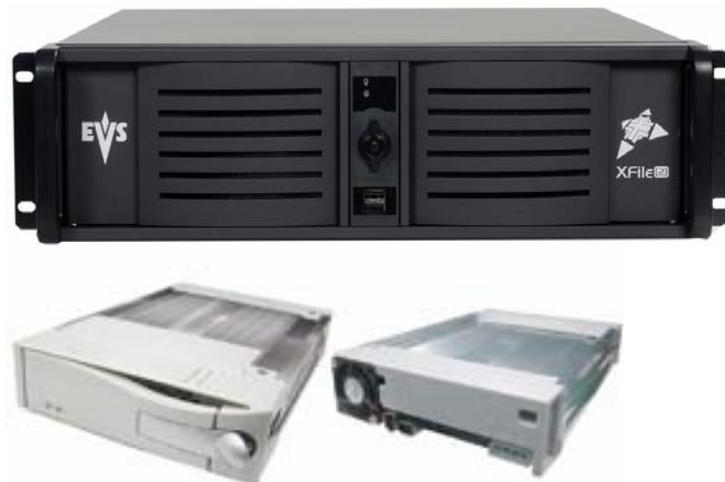
The XFILE platform is included in the XNet in which XT6U, XT4U SpotBox and AirBox servers interact via SDTI network.
