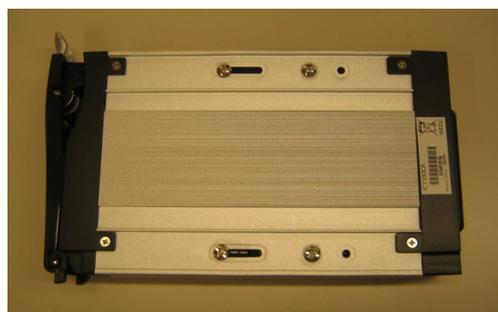
3. Place the disk tray cover, and then insert it into the XF2.
