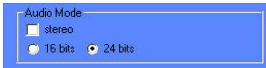
Selecting the **Stereo** option results in grouping server's mono channels in stereo channels.
