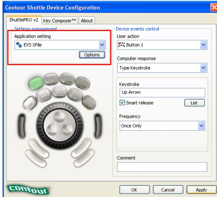
5. Click **APPLY** to confirm that the XFile settings are to be applied to the ShuttlePRO.
