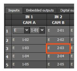
The E2-03 value located in the intersection between row 3 and column IN2 means that the 3<sup>rd</sup> audio mono channel of the embedded audio source plugged into the IN2 (CAMB) connector will be recorded on the same position on the EVS server.
