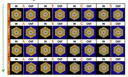
The record channels (IN connectors) are always assigned from bottom to top, whether working in UHD-4K or HD.
