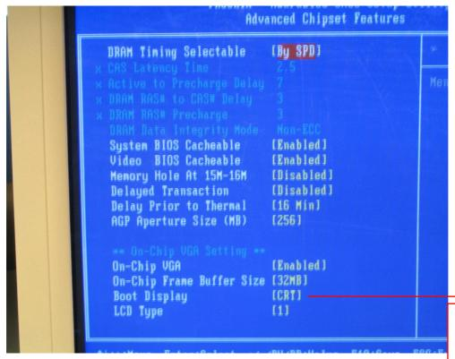
Can be changed to LCD&CRT depending of the monitor
