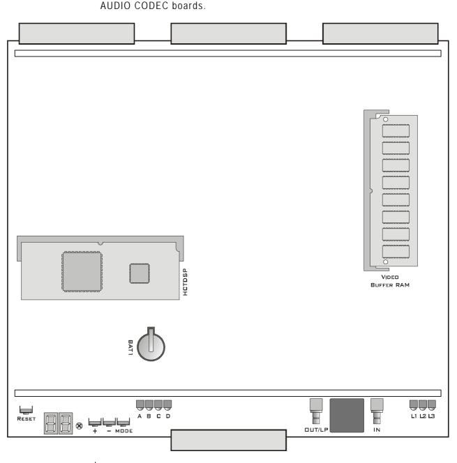
*Note:* The RESET button resets the board itself and initialises the RAM Video Buffer.
