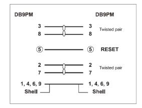
The RS 422 cable of the Remote control panel must be wired PIN TO PIN following the above diagram. Use shielded cable to avoid electromagnetic interference on long distances.
