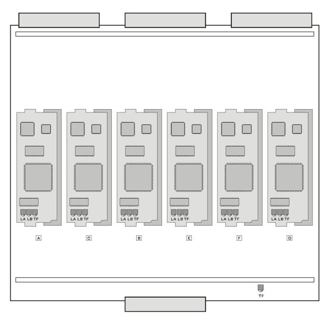
One CODEC module provides one video channel. Up to 6 modules can be plugged onto the VIDEO CODEC board, so the maximum configuration is 6-channel.
