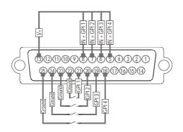
3.5.2 RELAY  $\rightarrow$  TTL INPUTS ON THE XT SERVER (GPI INPUTS 5, 6, 7, 8)
