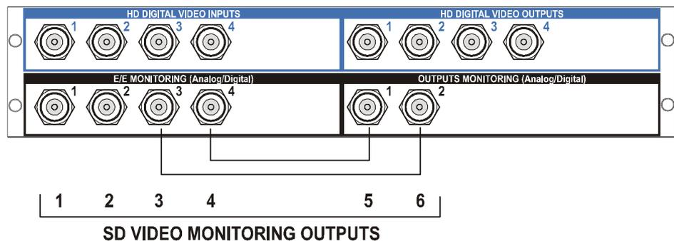
SD outputs assignment on 2-ch XT HD server when set to Monitoring only :
