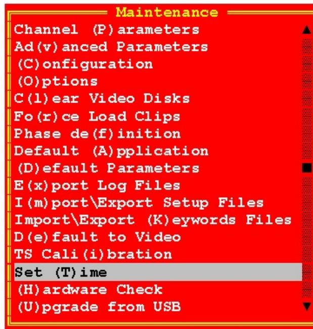
To select an option, use the <↑> and <↓> keys of the keyboard to highlight the corresponding line and press <ENTER> or press the key corresponding to the character between brackets.
