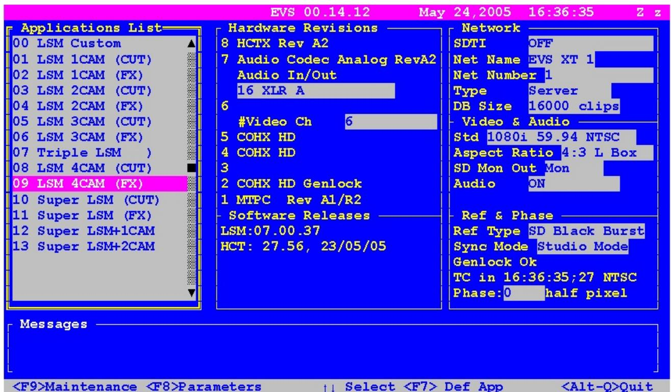
To enter the configuration window, press <F9> to open the Maintenance menu, select 'Configuration' and press <ENTER>. A double frame appears around the Configuration window, and the cursor blinks next to the 'HCT' label.
