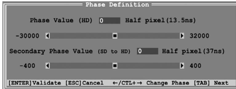
The main phase value for HD can be adjusted between - 30000 ns and +32000 ns by 13.5 ns steps and the secondary phase value (relative phase of the SD SDI outputs compared to the phase of the HD SDI outputs) can be adjusted between - 400 ns and +400 ns by 37ns steps
