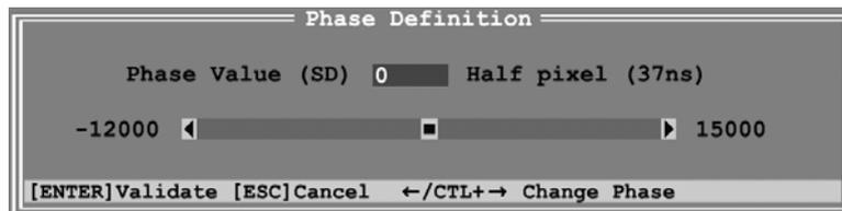
The phase value for SD can be adjusted between - 12000 ns and +15000 ns by 37 ns steps.
