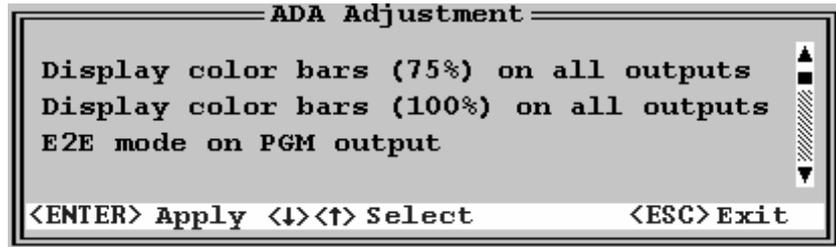
The E2E mode (Live) displays one input on the PGM output. So the video signal passes through the disk recorder system and through the ADA converters.
