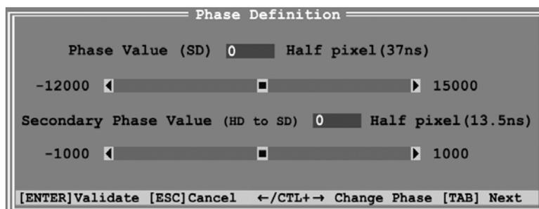
The main phase value for SD can be adjusted between - 12000 ns and +15000 ns by 37 ns steps and the secondary phase value (relative phase of the HD SDI outputs compared to the phase of the SD SDI outputs) can be adjusted between - 1000 ns and +1000 ns by 13.5 ns steps
