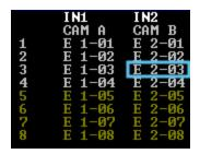
The E2-03 value located in the intersection between row 3 and column IN2 means that the 3<sup>rd</sup> audio mono channel of the embedded audio source plugged into the IN2 (CAMB) connector will be recorded on the same position on the EVS server.
