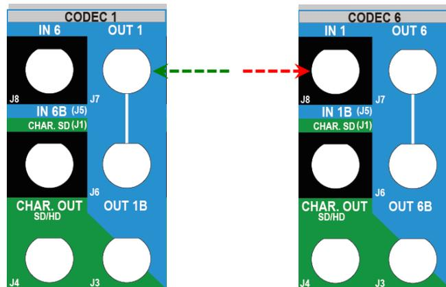
2. The **secondary links** of the V3X boards mentioned in the tables of this chapter correspond to the middle connectors of a codec module:
