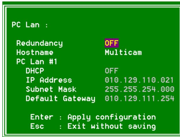
2. In this window, click **TAB** to select the **Redundancy** field, and press the **Space** bar to enable or disable the redundancy.
