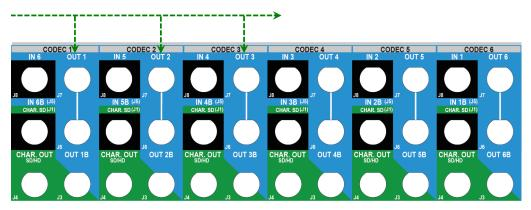
• The record channels (IN connectors) are always assigned from the right to the left.
